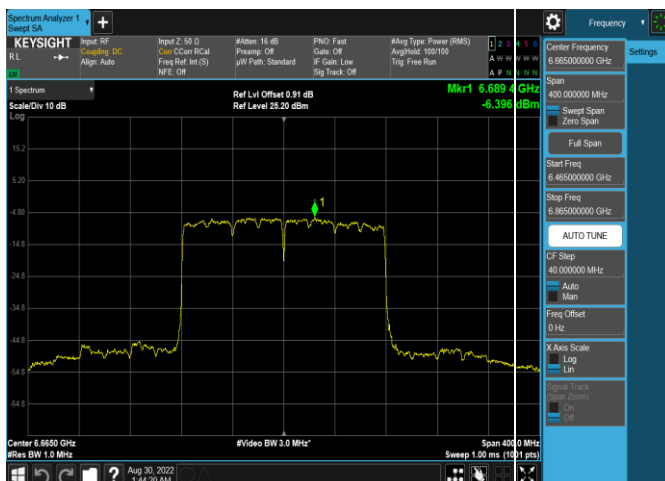
Plot 7-155. Power Spectral Density Plot Antenna 5b (160MHz 802.11ax (UNII Band 7) – Ch. 143, MCS4)
