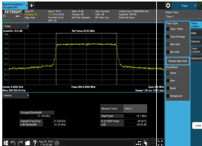
Plot 7-119. 26dB & 99% Bandwidth Plot Antenna 4a (80MHz 802.11ax (UNII Band 8) – Ch. 199, MCS11)
