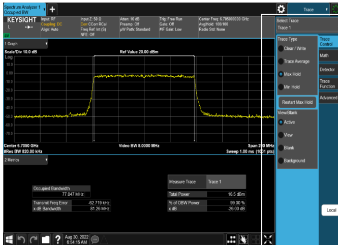
Plot 7-114. 26dB & 99% Bandwidth Plot Antenna 4a (80MHz 802.11ax (UNII Band 7) – Ch. 151, MCS11)
