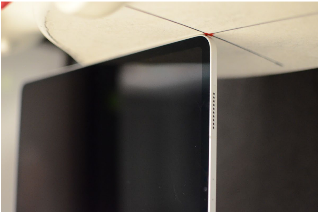
SAR Test Setup Photo 12: Left Edge at 0.0 cm – Ant 3/4a/4b
