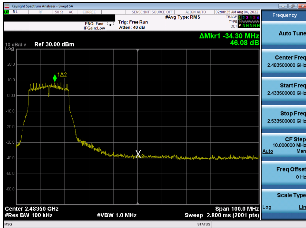
Plot 7-217. Band Edge Plot Antenna 4a (802.11g- Ch. 8) – 18Mbps
