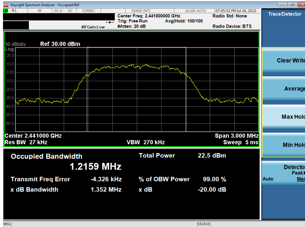
Plot 7-5. 20dB BW and 99% OBW Plot Antenna 4a (Bluetooth, 8DPSK, ePA – 2441 MHz)
