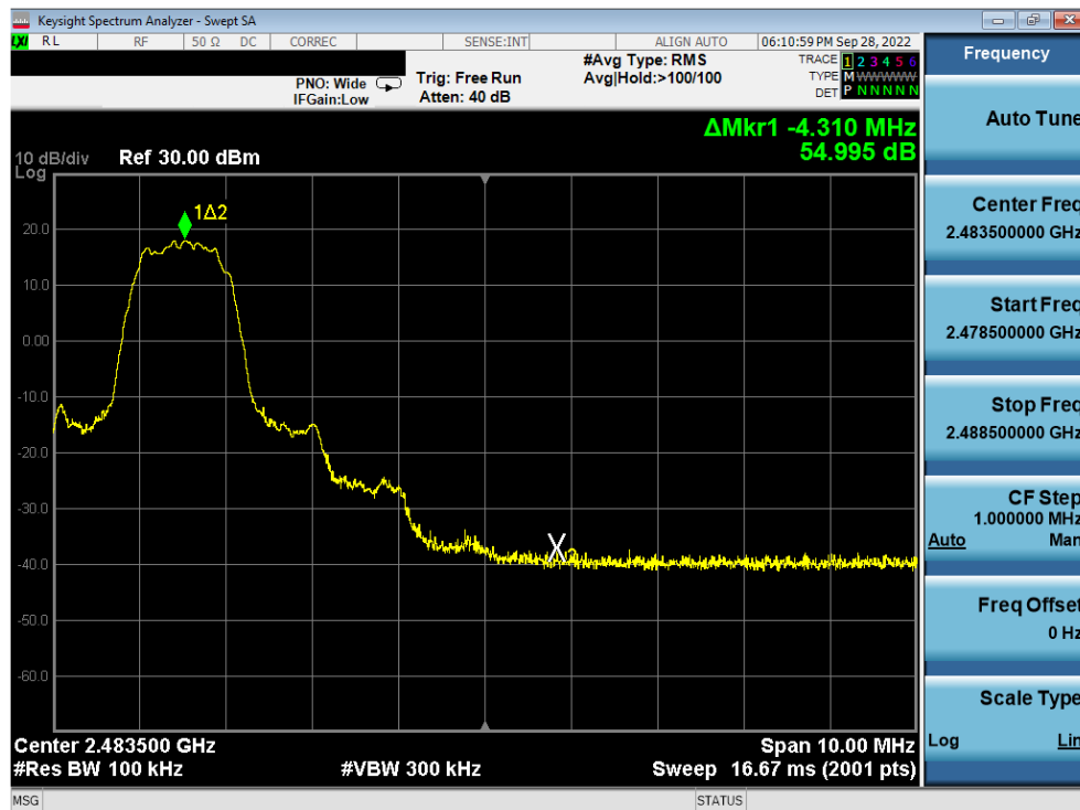
Plot 7-18. Band Edge Plot Antenna 4a (Bluetooth with Hopping Disabled, 8DPSK, ePA – 2480 MHz)
