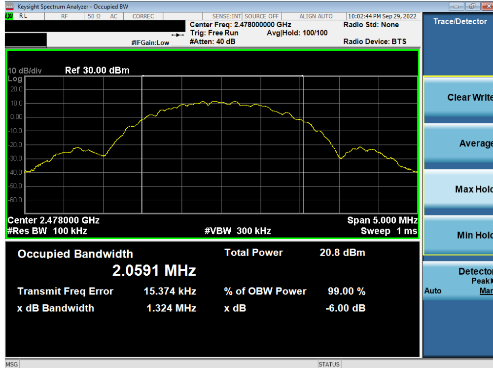
Plot 7-12. 6dB BW & 99% OBW Antenna 2a (Bluetooth (LE), 2Mbps, ePA – Ch. 38)
