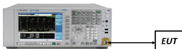
Figure 7-4. Test Instrument & Measurement Setup
