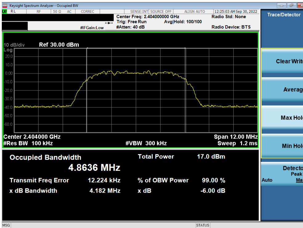
Plot 7-10. 6dB BW & 99% OBW Plot Antenna 2a (Bluetooth (HDR8), 8Mbps, ePA – Ch. 1)
