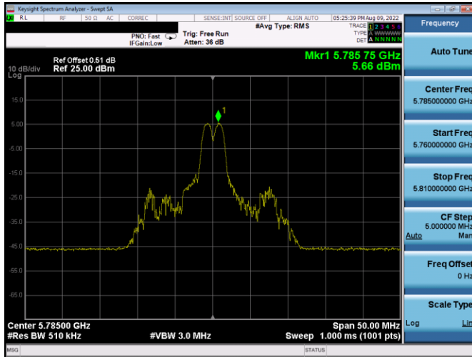
Plot 7-158. PSD Antenna WF5b (20MHz BW 11ax Index 4 – RU26 – Ch.157)
