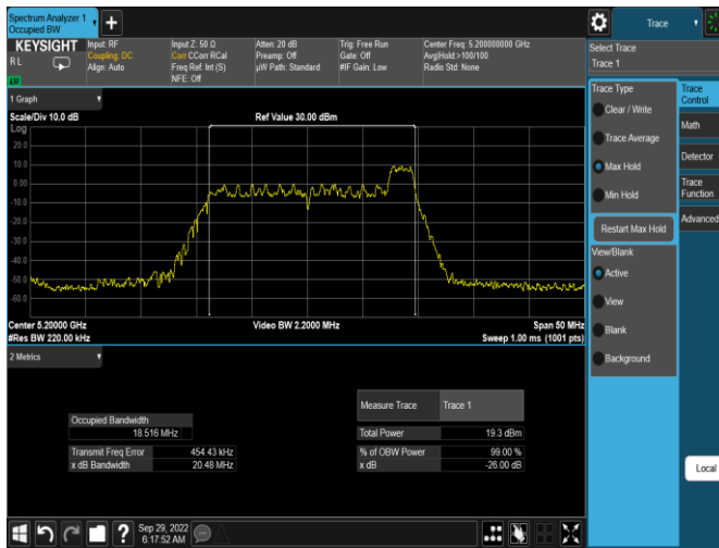
Plot 7-3. 26dB BW & 99% OBW Antenna WF5b (20MHz BW 11ax Index 8– RU26 – Ch.40)
