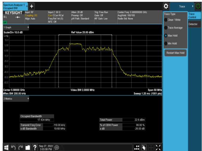
Plot 7-30. 26dB BW & 99% OBW Antenna WF5b (20MHz BW 11ax Index 38 – RU52 – Ch.116)
