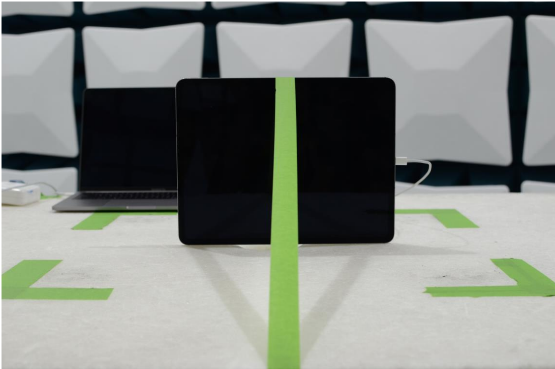
Figure 15: 30MHz-1GHz Test Setup (Front View)
