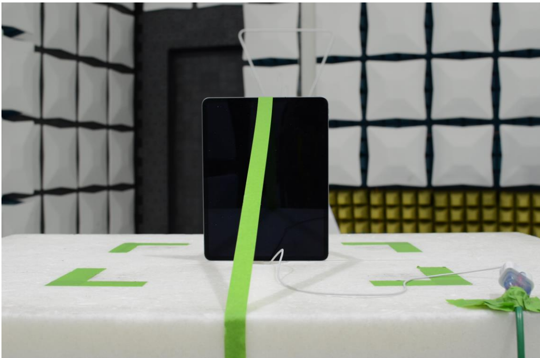
Figure 12: 30MHz-1GHz Test Setup (Rear View)
