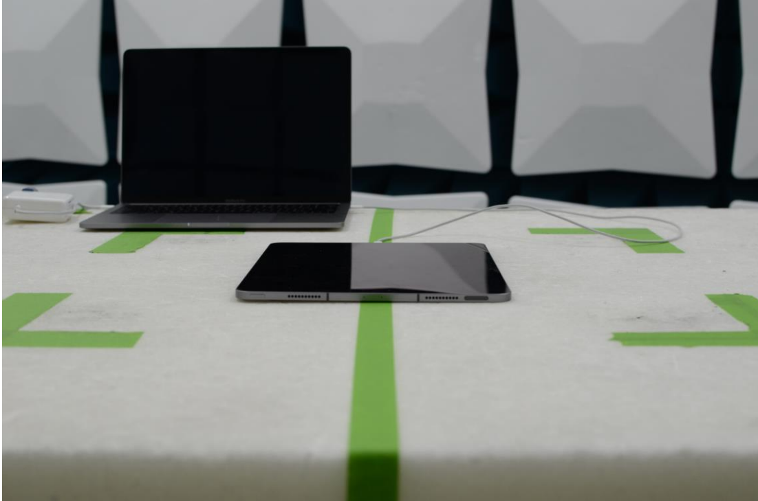
Figure 13: 30MHz-1GHz Test Setup (Front View)
