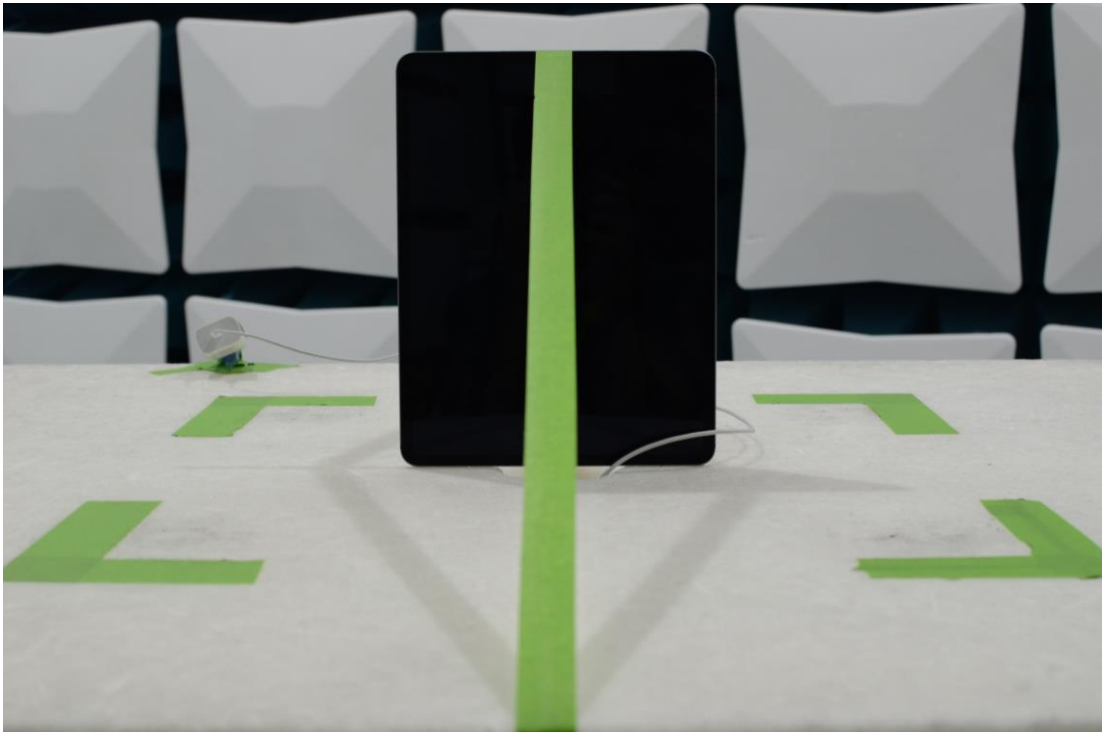
Figure 11: 30MHz-1GHz Test Setup (Front View)
