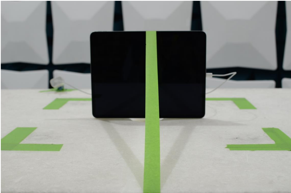
Figure 9: 30MHz-1GHz Test Setup (Front View)
