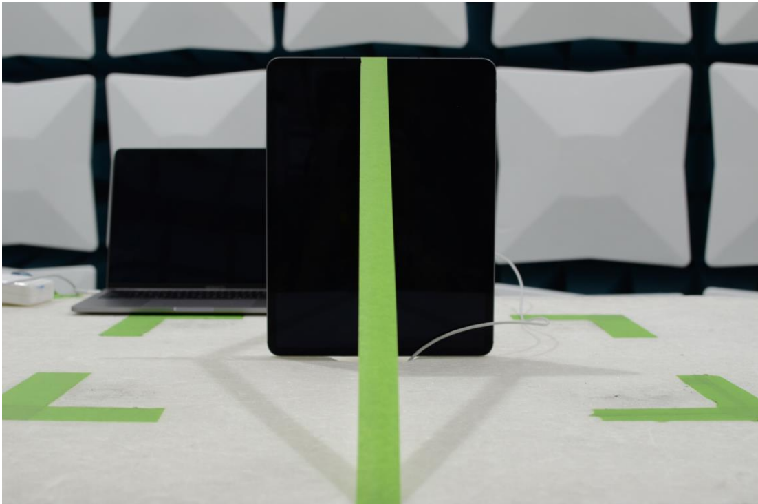
Figure 17: 30MHz-1GHz Test Setup (Front View)
