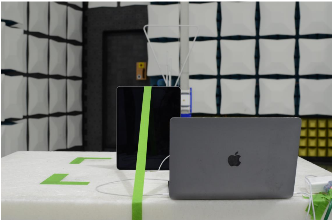
Figure 18: 30MHz-1GHz Test Setup (Rear View)
