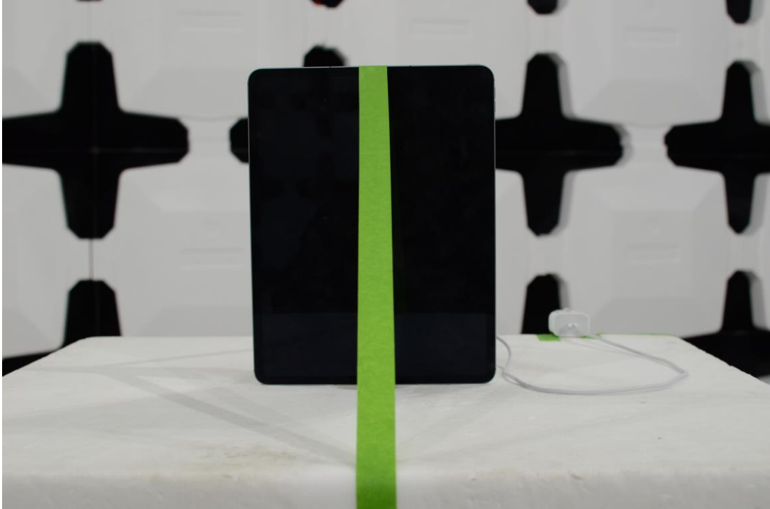
Figure 5: 1-18GHz Test Setup (Front View)
