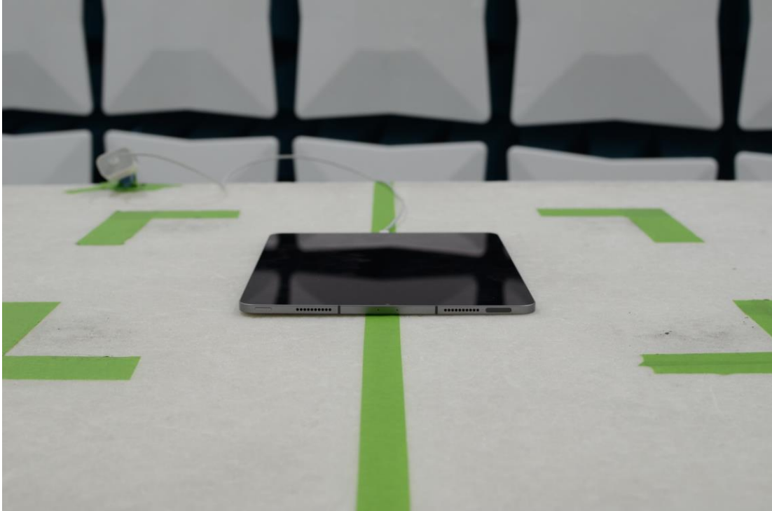
Figure 7: 30MHz-1GHz Test Setup (Front View)
