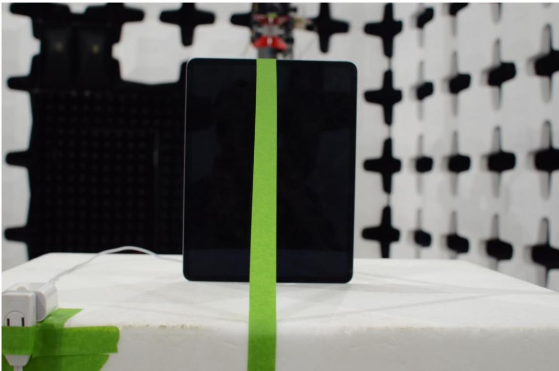
Figure 6: 1-18GHz Test Setup (Rear View)
