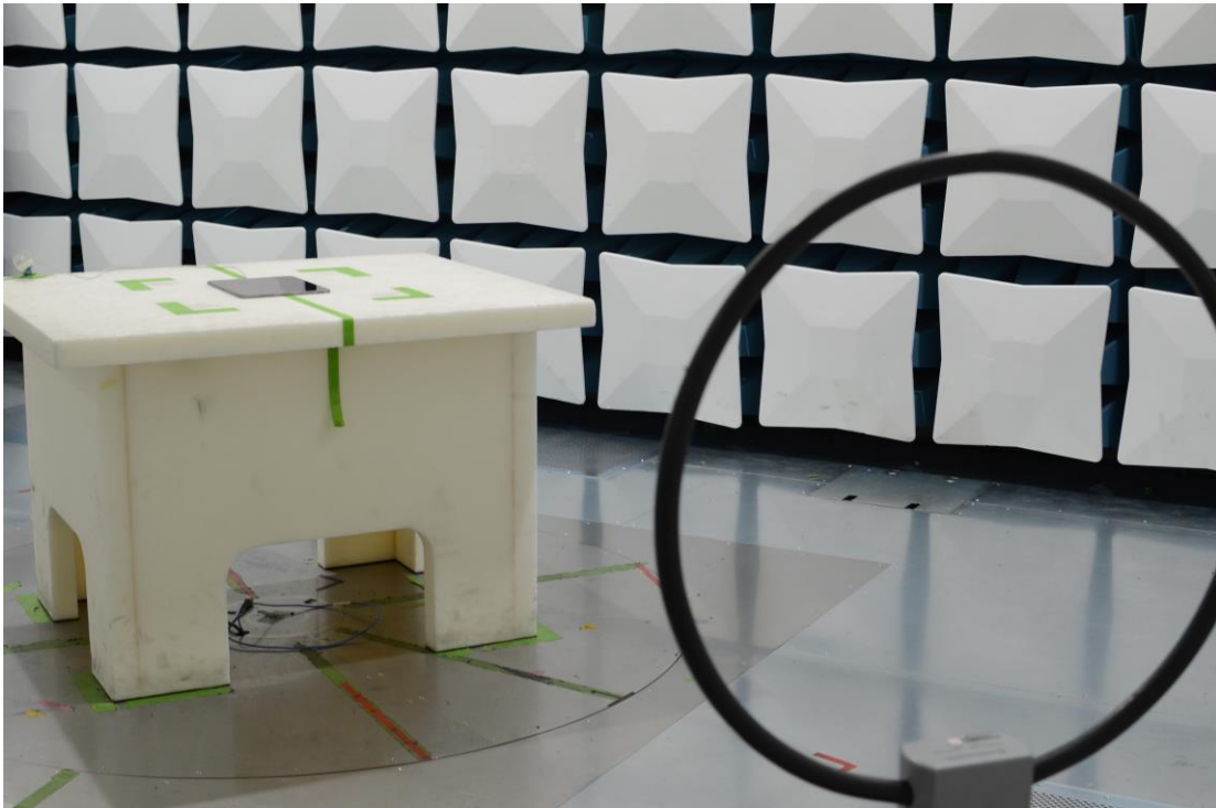
Figure 19: 9kHz-30MHz Test Setup (Front View)
