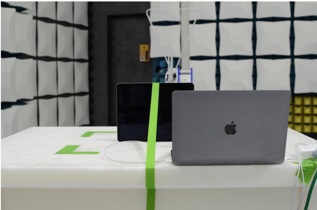
Figure 16: 30MHz-1GHz Test Setup (Rear View)
