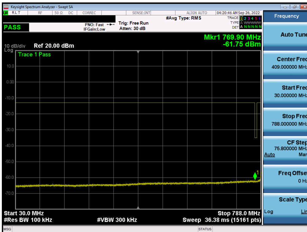
Plot 7-57. Conducted Spurious Plot (LTE Band 14 - 10MHz QPSK - RB Size 1, RB Offset 0 - Mid Channel)
