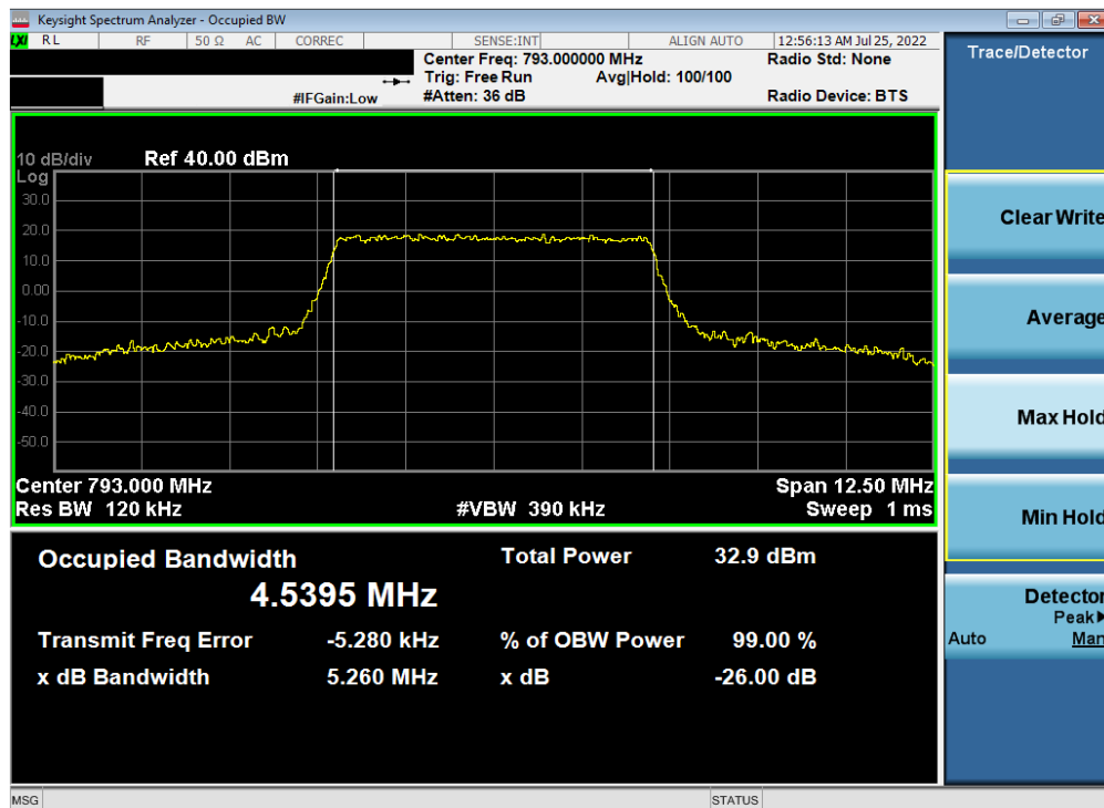
Plot 7-18. Occupied Bandwidth Plot (LTE Band 14 - 5MHz 16-QAM - Full RB Configuration)
