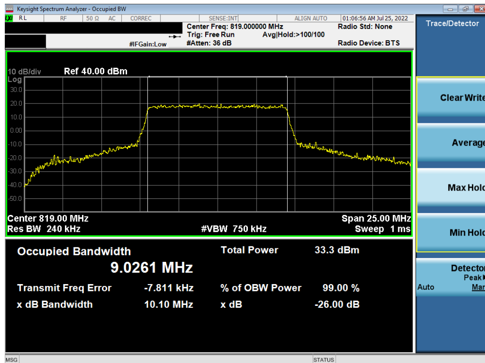
Plot 7-14. Occupied Bandwidth Plot (LTE Band 26 - 10MHz 16-QAM - Full RB Configuration)
