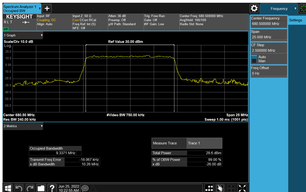
Plot 7-119. Occupied Bandwidth Plot (NR Band n71 - 10MHz CP-OFDM 256-QAM - Full RB)
