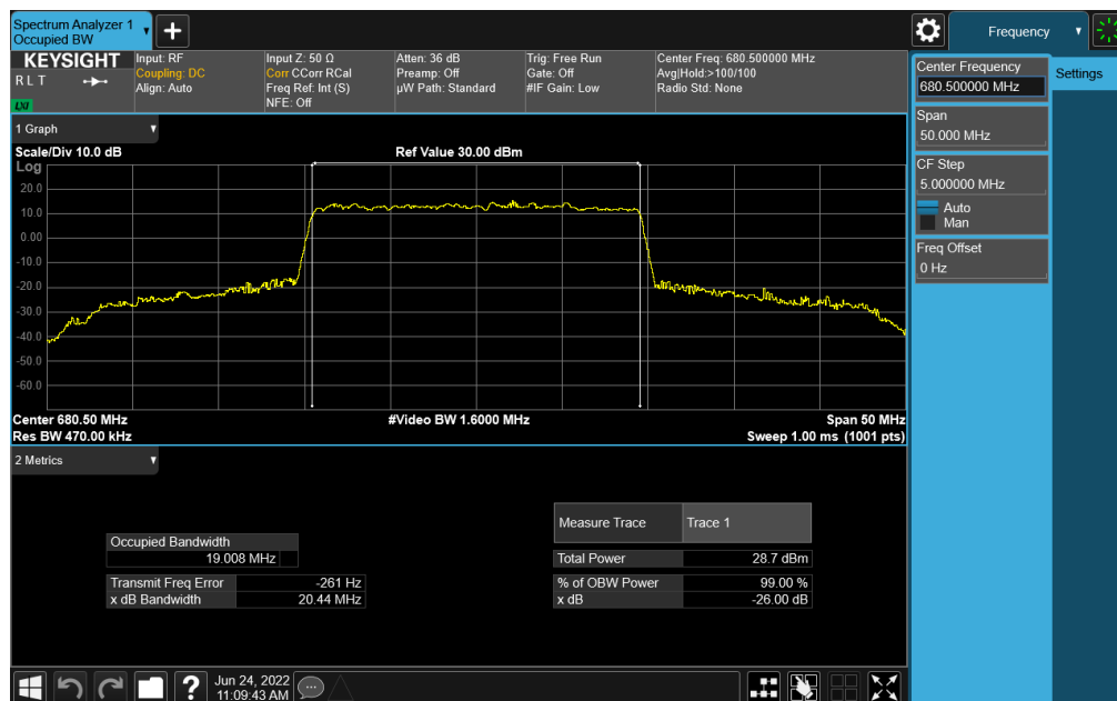
Plot 7-129. Occupied Bandwidth Plot (NR Band n71 - 20MHz CP-OFDM 256-QAM - Full RB)
