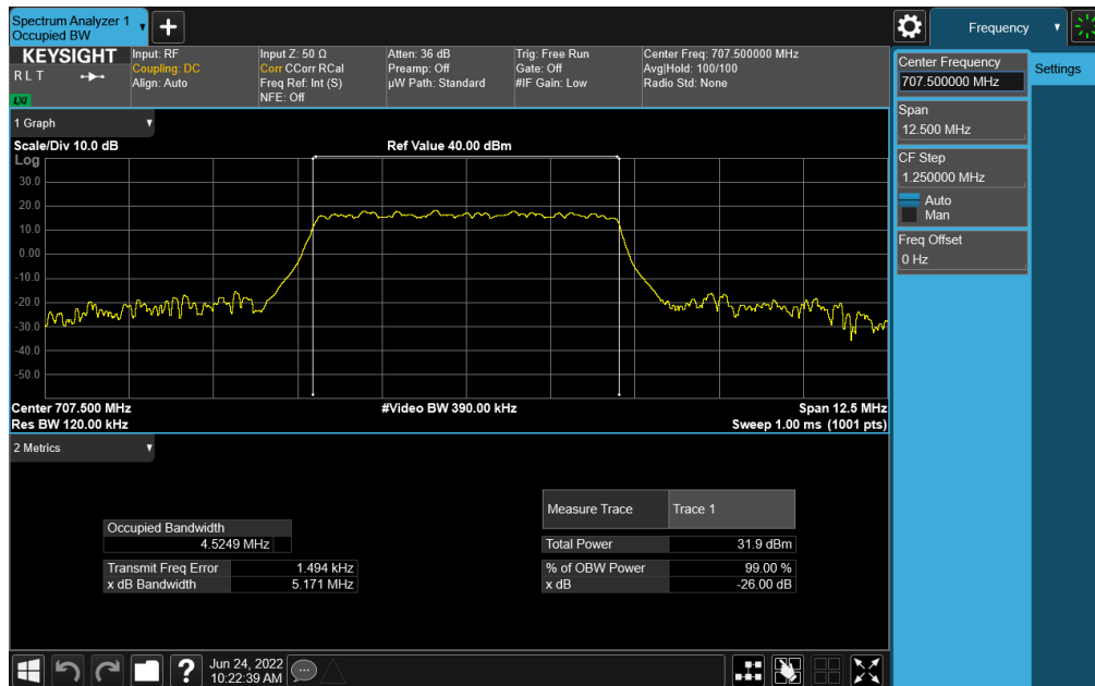
Plot 7-132. Occupied Bandwidth Plot (NR Band n12 - 5MHz DFT-s-OFDM 16-QAM - Full RB)
