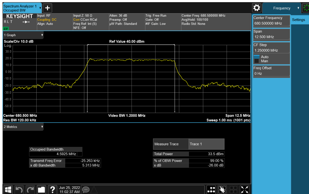
Plot 7-110. Occupied Bandwidth Plot (NR Band n71 - 5MHz DFT-s-OFDM \pi/2 BPSK - Full RB)
