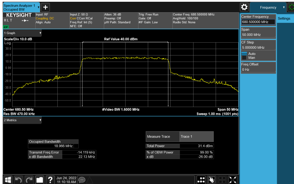
Plot 7-128. Occupied Bandwidth Plot (NR Band n71 - 20MHz CP-OFDM 64-QAM - Full RB)
