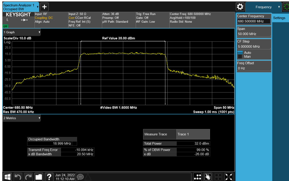
Plot 7-126. Occupied Bandwidth Plot (NR Band n71 - 20MHz CP-OFDM QPSK - Full RB)
