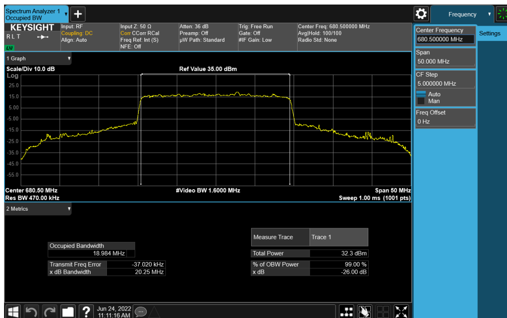
Plot 7-127. Occupied Bandwidth Plot (NR Band n71 - 20MHz CP-OFDM 16-QAM - Full RB)
