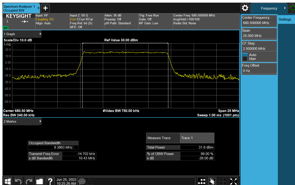
Plot 7-117. Occupied Bandwidth Plot (NR Band n71 - 10MHz CP-OFDM 16-QAM - Full RB)
