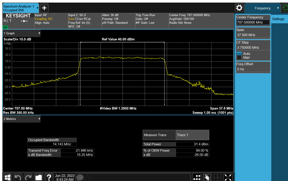
Plot 7-143. Occupied Bandwidth Plot (NR Band n12 - 15MHz CP-OFDM 64-QAM - Full RB)
