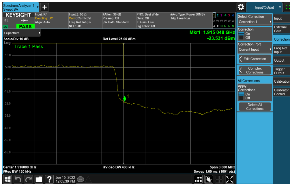
Plot 7-142. Upper Band Edge Plot (NR Band n25 – 10MHz DFT-s-OFDM \pi/2 BPSK – Full RB Configuration)
