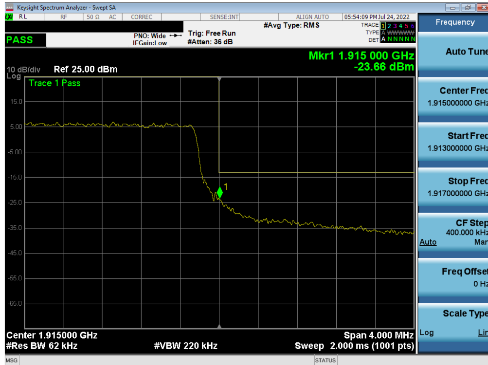
Plot 7-98. Upper Band Edge Plot (LTE Band 25 – 5MHz QPSK – Full RB Configuration)
