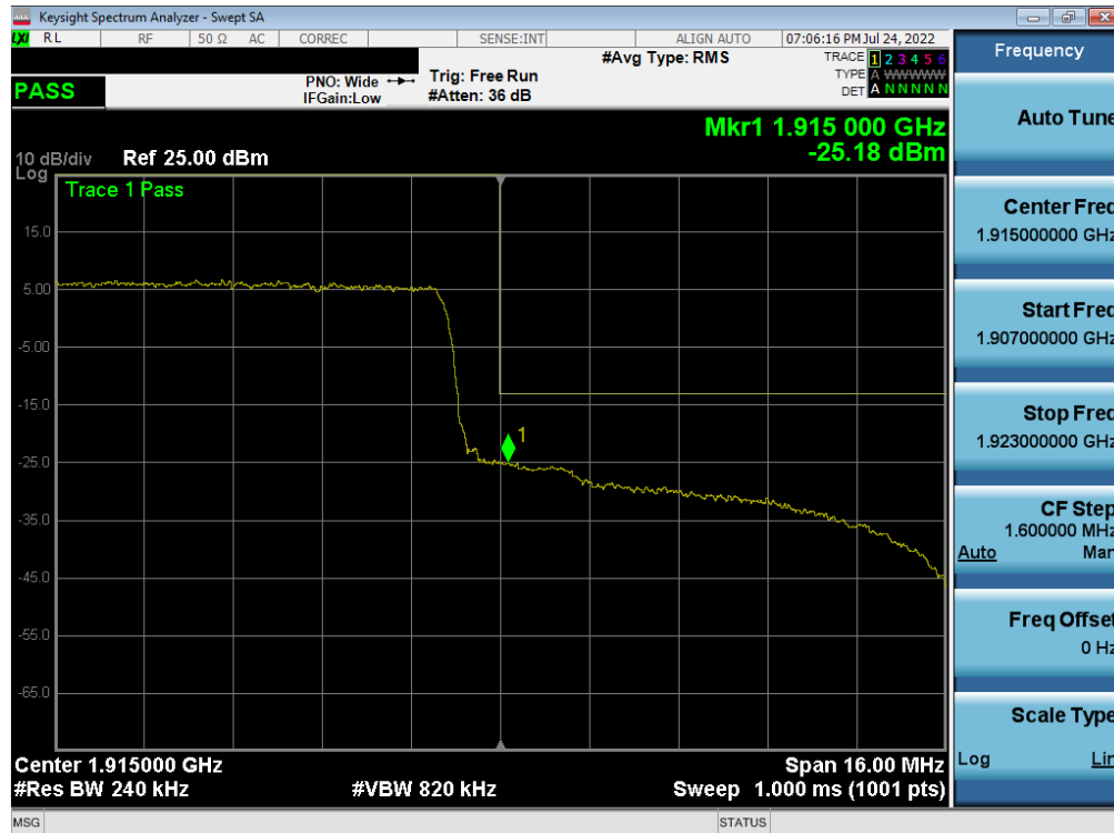
Plot 7-110. Upper Band Edge Plot (LTE Band 25 – 20MHz QPSK – Full RB Configuration)
