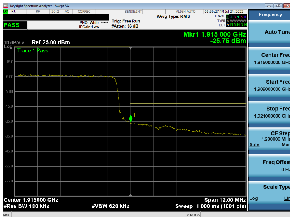
Plot 7-106. Upper Band Edge Plot (LTE Band 25 – 15MHz QPSK – Full RB Configuration)
