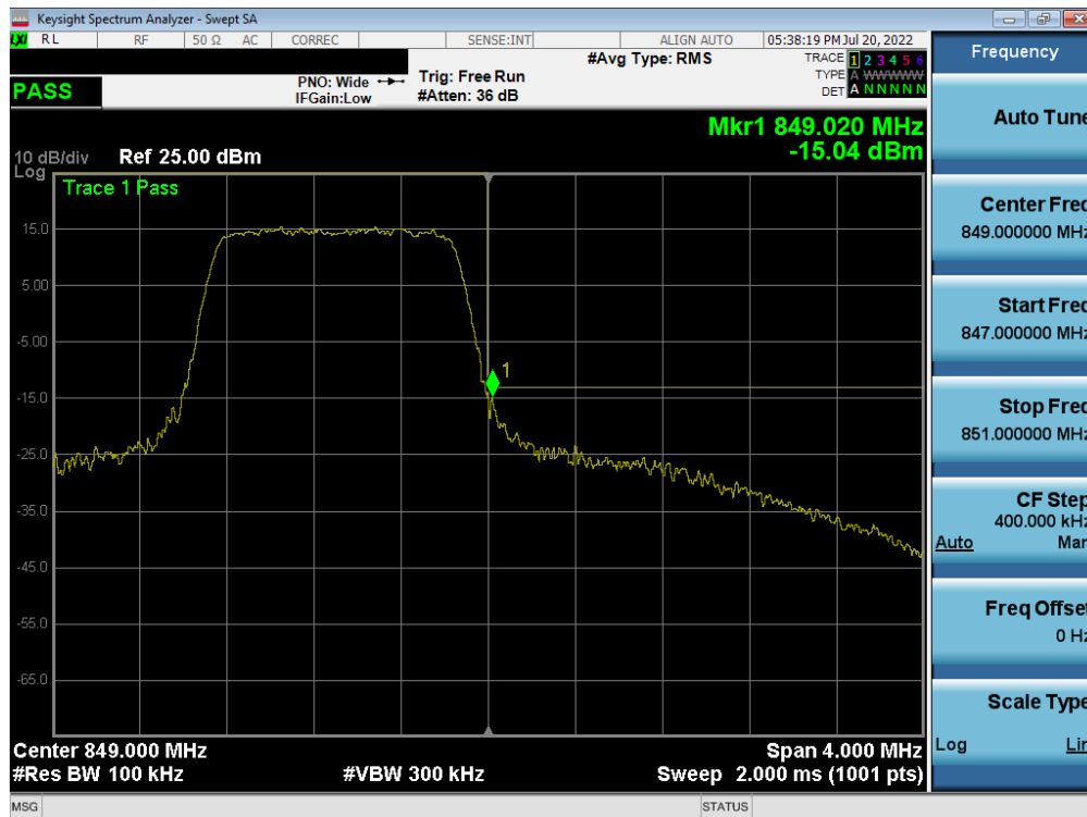
Plot 7-93. Upper BE Plot (LTE Band 5 – 1.4MHz QPSK – Full RB Configuration)
