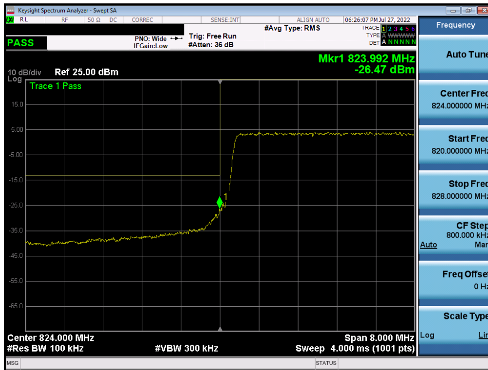
Plot 7-104. Lower BE Plot (NR Band n26 DFT-s-OFDM - 10.0MHz - Full RB)
