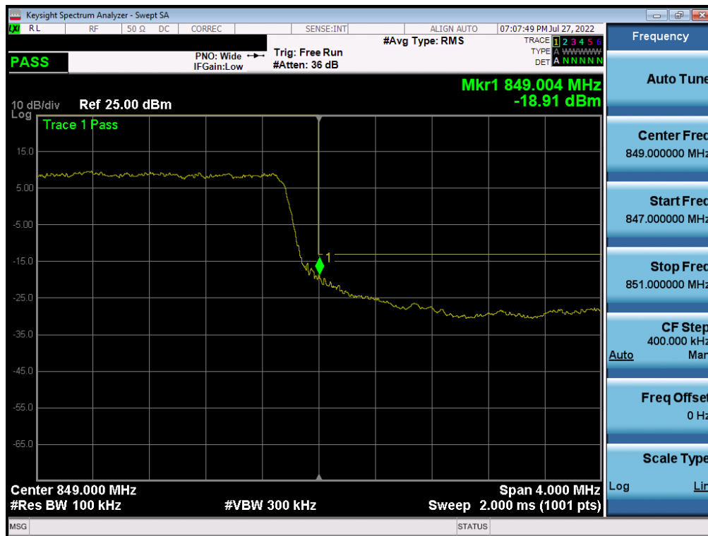
Plot 7-103. Upper BE Plot (NR Band n26 DFT-s-OFDM – 5.0MHz - Full RB)
