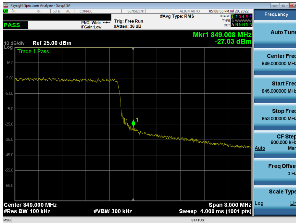
Plot 7-99. Upper BE Plot (LTE Band 5 - 10MHz QPSK – Full RB Configuration)
