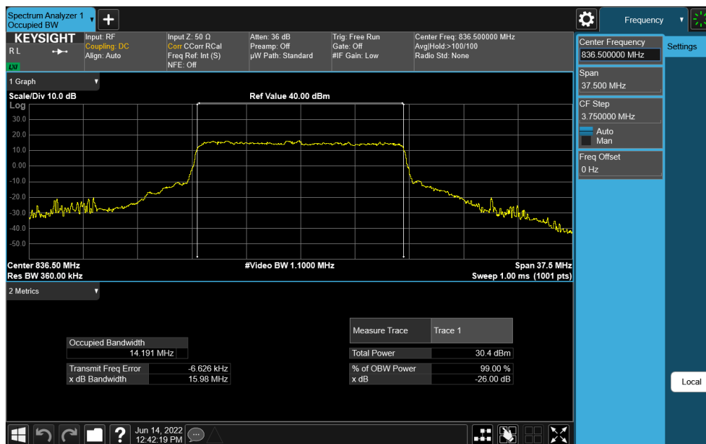
Plot 7-30. Occupied Bandwidth Plot (NR Band n5 - CP-OFDM 15MHz 64-QAM - Full RB Configuration)
