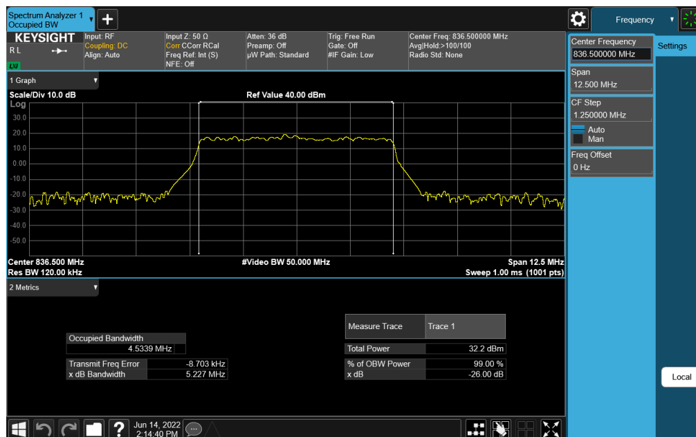
Plot 7-18. Occupied Bandwidth Plot (NR Band n26/5 - DFT-s-OFDM 5MHz QPSK - Full RB Configuration)
