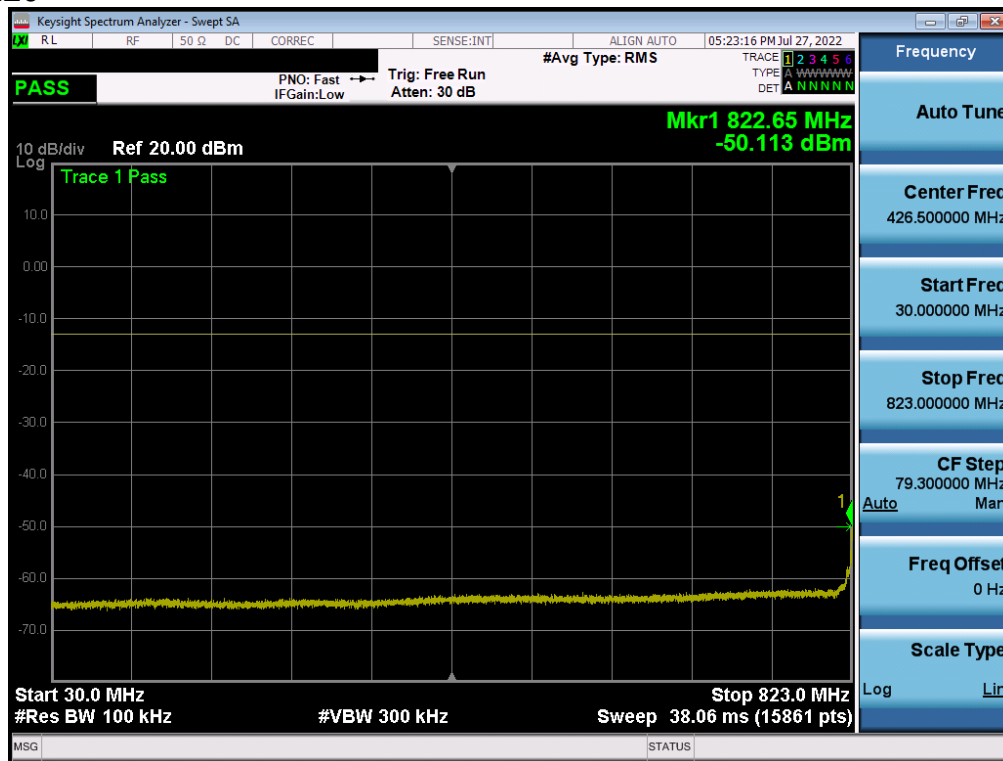
Plot 7-66. CSE (NR Band n26 - 10.0MHz DFT-s-OFDM QPSK - RB Size 1, RB Offset 0 - Low Channel)
