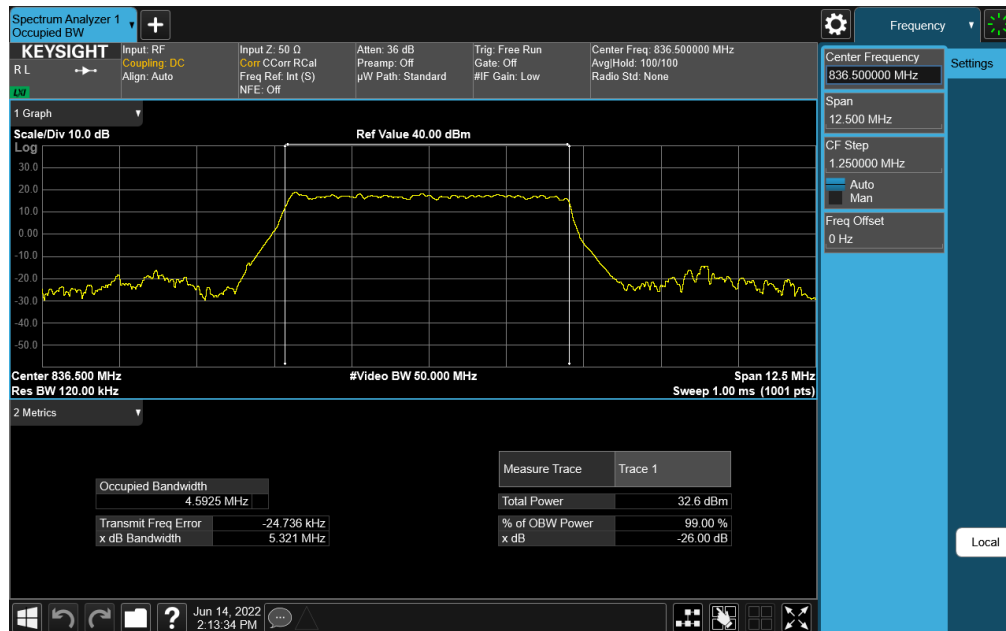
Plot 7-17. Occupied Bandwidth Plot (NR Band n26/5 - 5MHz DFT-s-OFDM \pi/2 BPSK - Full RB Configuration)
