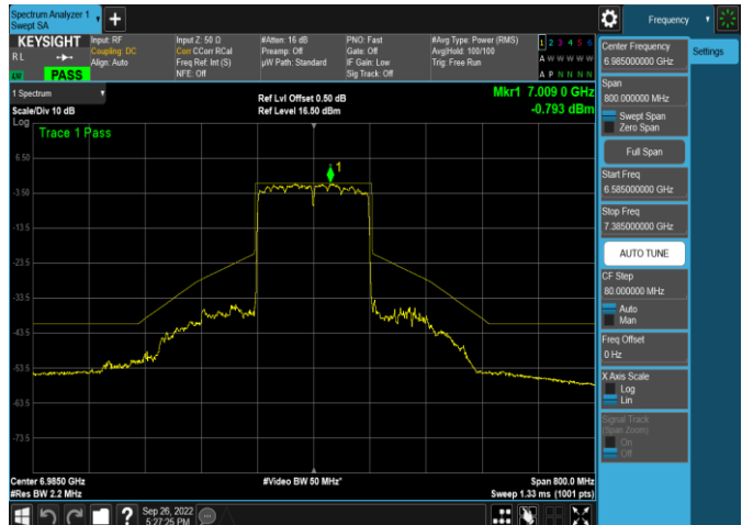
Plot 7-447. In-Band Emission Plot Antenna WF5t (160MHz 802.11ax RU484 (UNII Band 8) – Ch. 207)
