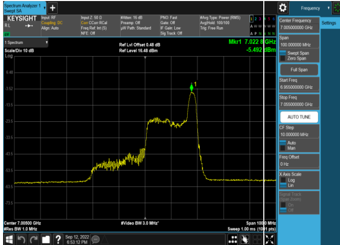
Plot 7-247. Power Spectral Density Plot Antenna WF5b (40MHz 802.11ax RU26 (UNII Band 8) - Ch. 211)
