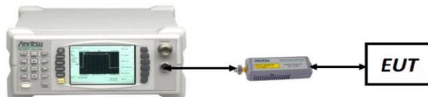
Figure 7-2. Test Instrument & Measurement Setup
