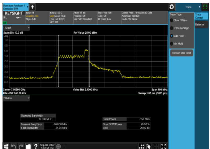
Plot 7-54. 26dB & 99% Bandwidth Plot Antenna WF5t (40MHz 802.11ax RU26 (UNII Band 8) - Ch. 211)
