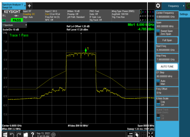
Plot 7-387. In-Band Emission Plot Antenna WF5t (160MHz 802.11ax (UNII Band 7) – Ch. 143, MCS11)
