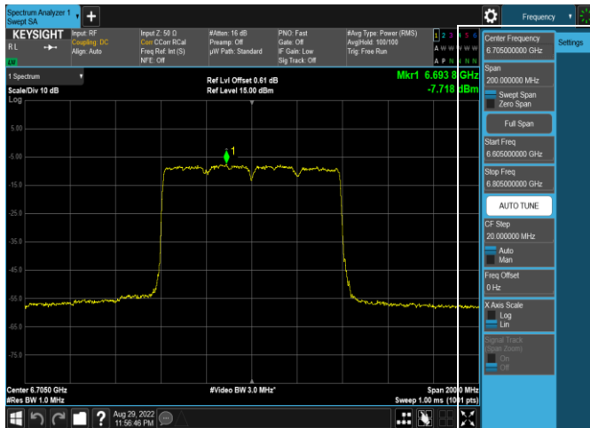
Plot 7-170. Power Spectral Density Plot Antenna WF5t (80MHz 802.11ax (UNII Band 7) – Ch. 151, MCS11)
