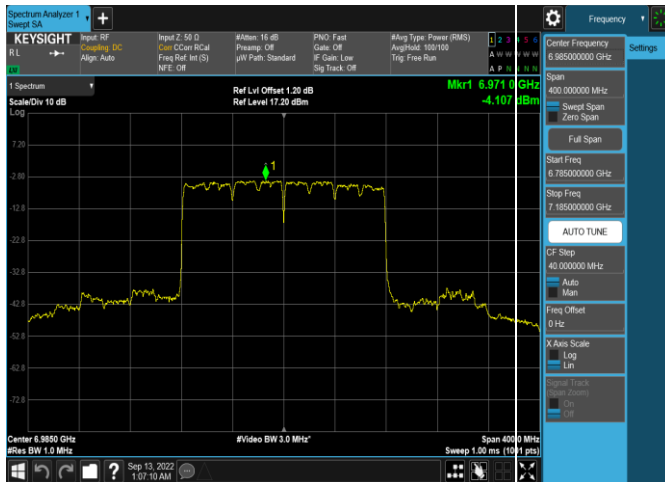
Plot 7-176. Power Spectral Density Plot Antenna WF5t (160MHz 802.11ax (UNII Band 8) – Ch. 207, MCS11)
