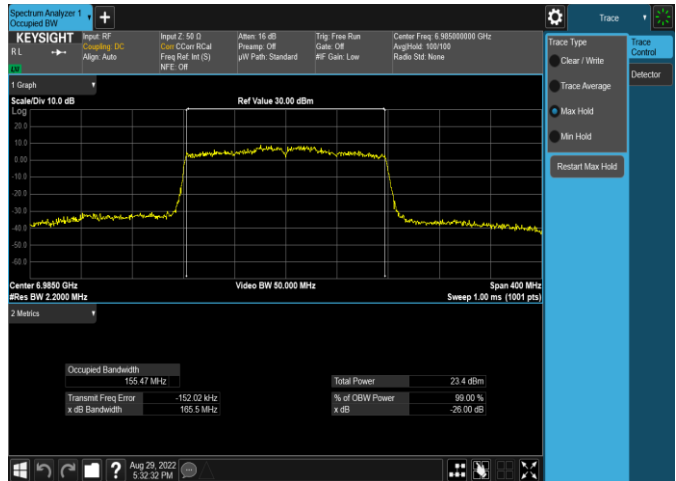
Plot 7-20. 26dB & 99% Bandwidth Plot Antenna WF5t (160MHz 802.11ax (UNII Band 8) – Ch. 207, MCS2)
