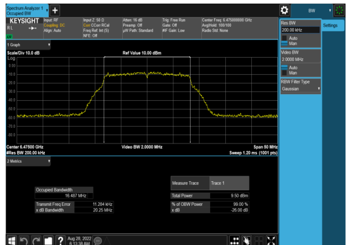
Plot 7-66. 26dB & 99% Bandwidth Plot Antenna WF5b (20MHz 802.11a (UNII Band 6) – Ch. 105, 12Mbps)
