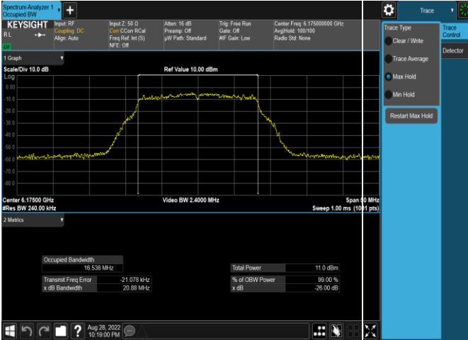
Plot 7-1. 26dB & 99% Bandwidth Plot Antenna WF5t (20MHz 802.11a (UNII Band 5) – Ch. 45, 12Mbps)
