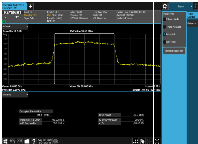
Plot 7-15. 26dB & 99% Bandwidth Plot Antenna WF5t (160MHz 802.11ax (UNII Band 7) – Ch. 143, MCS2)
