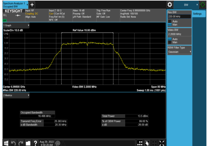
Plot 7-36. 26dB & 99% Bandwidth Plot Antenna WF5t (20MHz 802.11a (UNII Band 8) – Ch. 209, 24Mbps)
