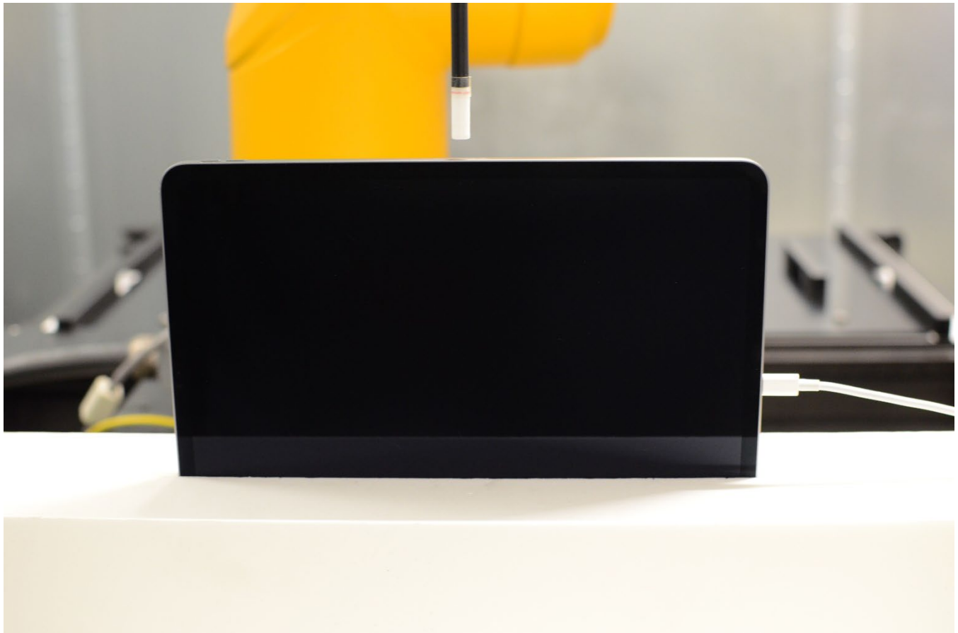
Figure F-11 Near Field Power Density Test Setup Photo – Right Edge at 8.58 mm
