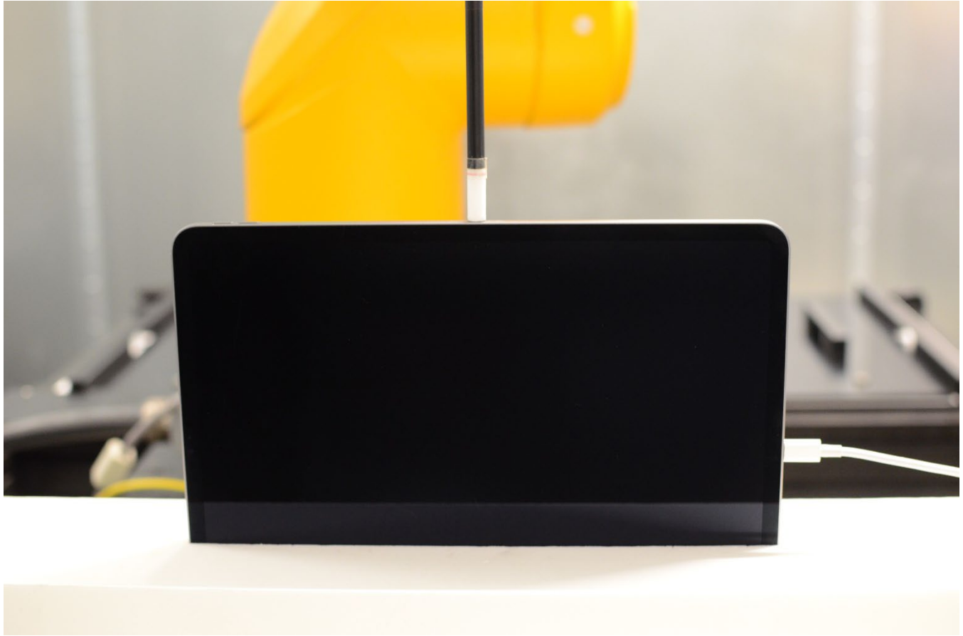
Figure F-10 Near Field Power Density Test Setup Photo – Right Edge at 2 mm
