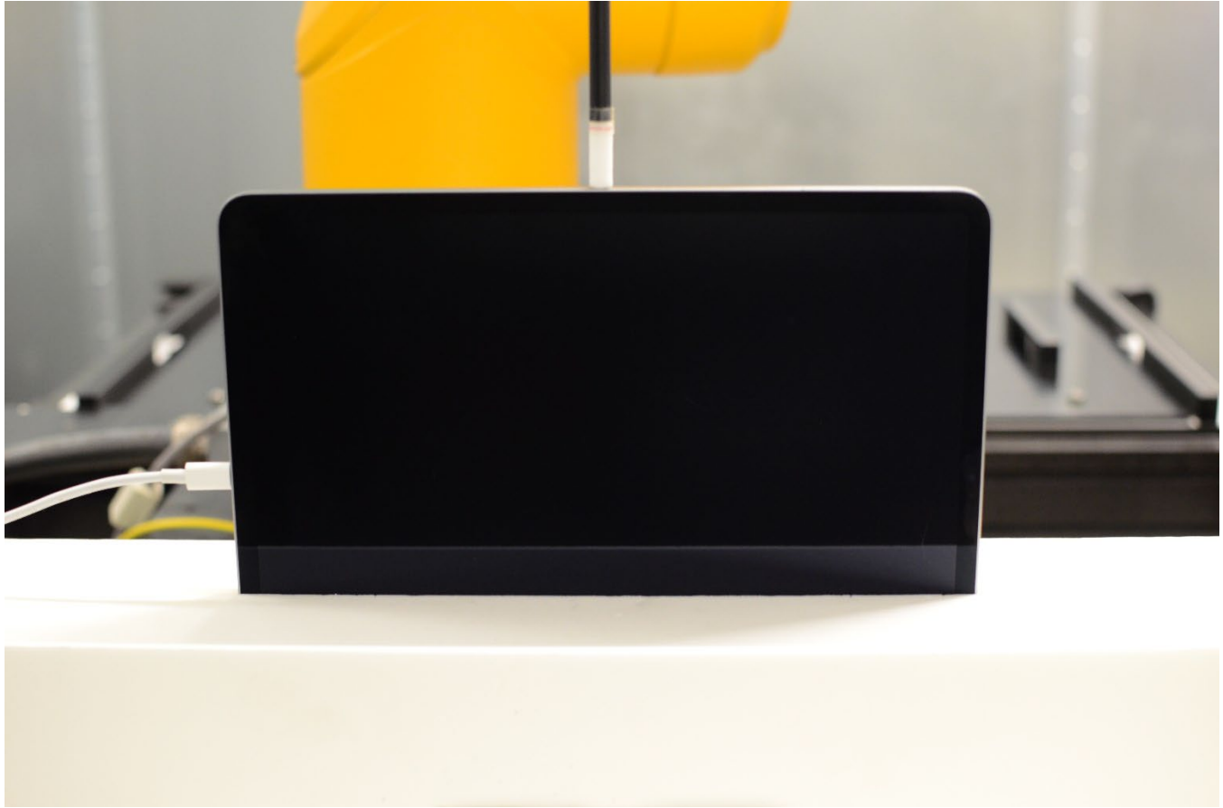
Figure F-12 Near Field Power Density Test Setup Photo – Left Edge at 2 mm
