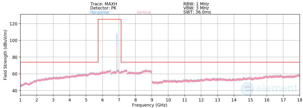
Plot 7-621. Radiated Spurious Emissions above 1GHz SDM (802.11ax – Ch. 185, MCS2)
