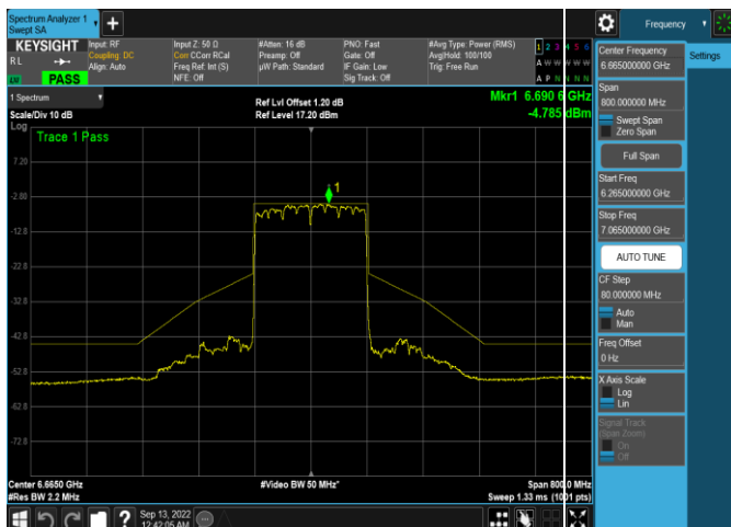
Plot 7-387. In-Band Emission Plot Antenna WF5t (160MHz 802.11ax (UNII Band 7) – Ch. 143, MCS11)
