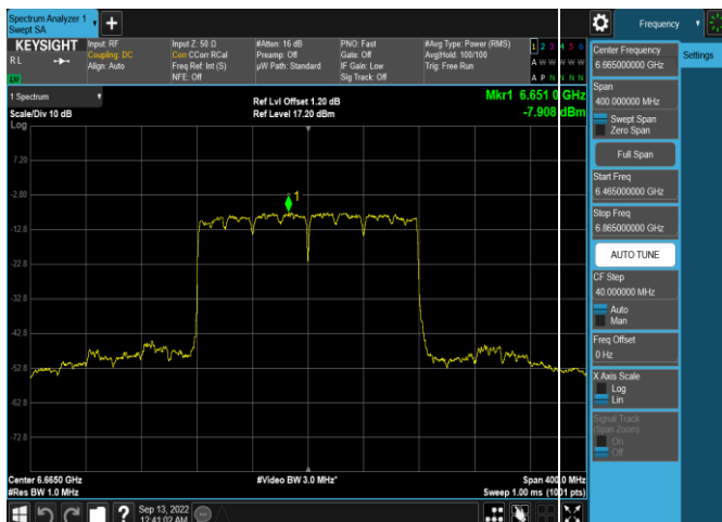
Plot 7-171. Power Spectral Density Plot Antenna WF5t (160MHz 802.11ax (UNII Band 7) – Ch. 143, MCS11)
