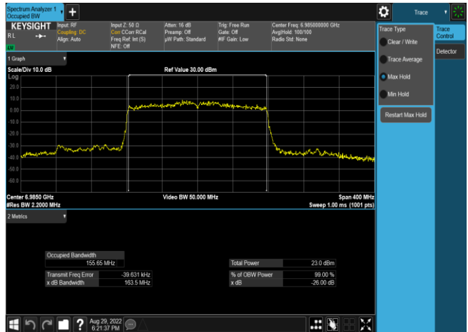
Plot 7-40. 26dB & 99% Bandwidth Plot Antenna WF5t (160MHz 802.11ax (UNII Band 8) – Ch. 207, MCS4)
