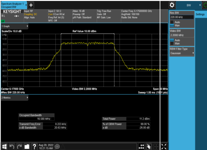
Plot 7-41. 26dB & 99% Bandwidth Plot Antenna WF5t (20MHz 802.11a (UNII Band 5) – Ch. 47, 54Mbps)
