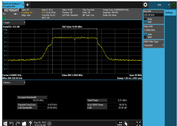
Plot 7-51. 26dB & 99% Bandwidth Plot Antenna WF5t (20MHz 802.11a (UNII Band 7) – Ch. 149, 54Mbps)
