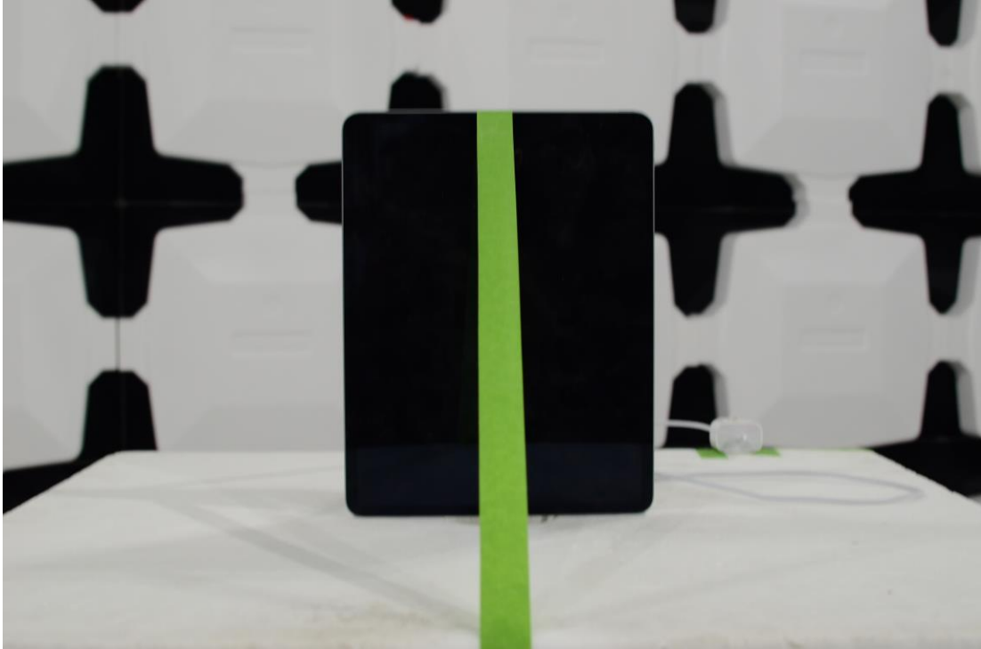
Figure 9: 1-18GHz Test Setup (Front View)
