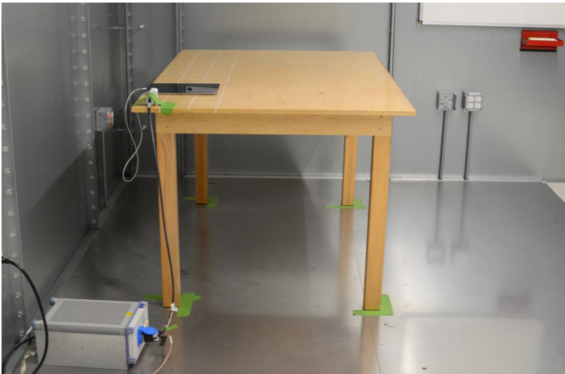
Figure 2: AC Line Conducted Emissions (Side View)
