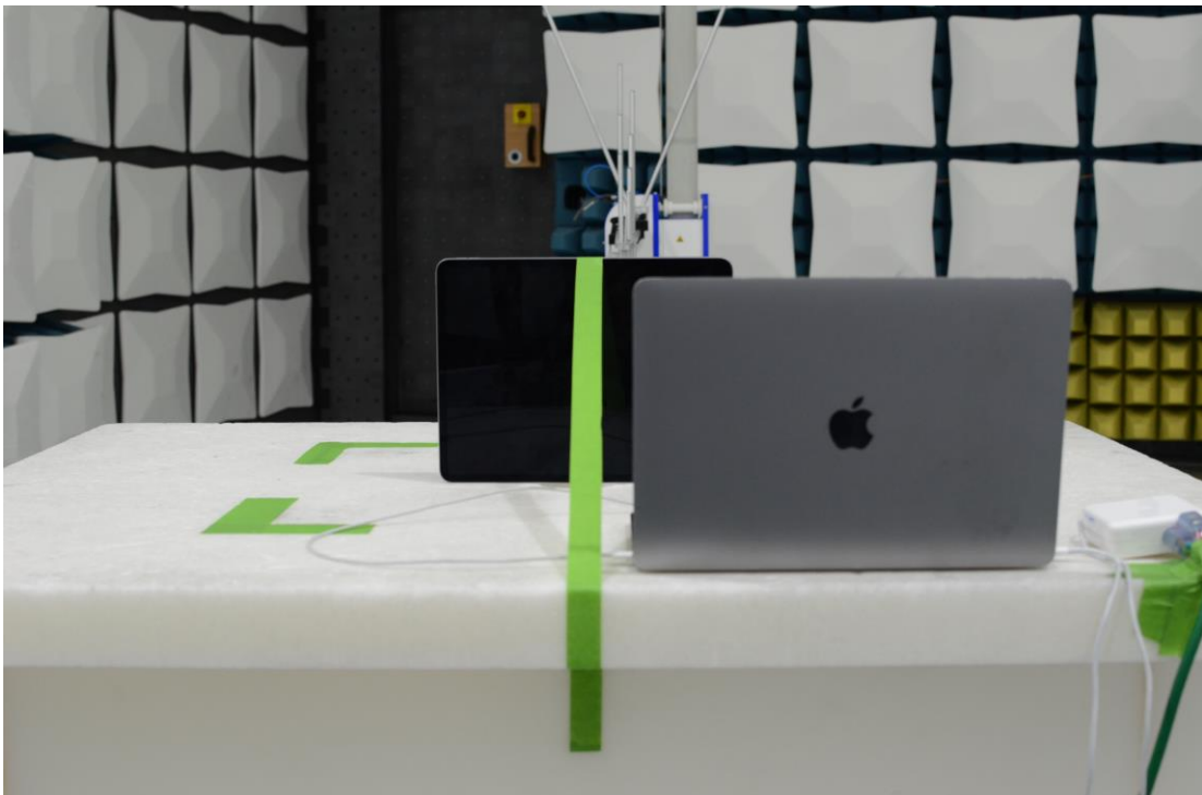
Figure 20: 30MHz-1GHz Test Setup (Rear View)
