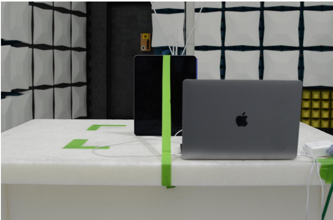
Figure 22: 30MHz-1GHz Test Setup (Rear View)
