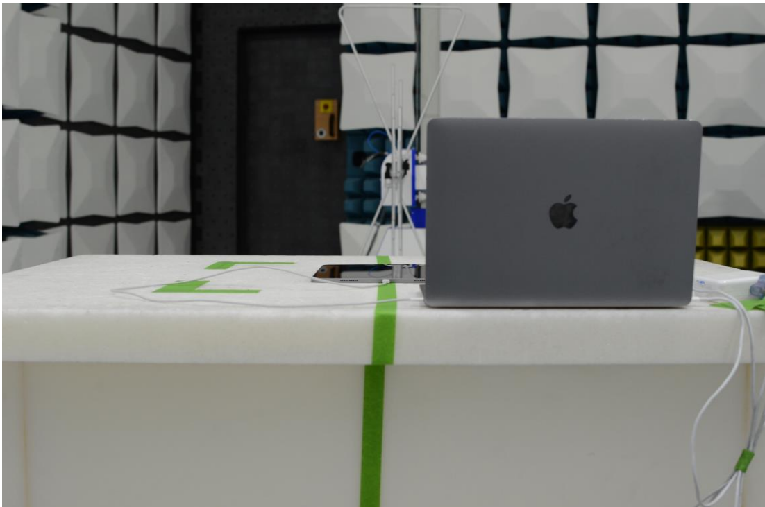
Figure 18: 30MHz-1GHz Test Setup (Rear View)
