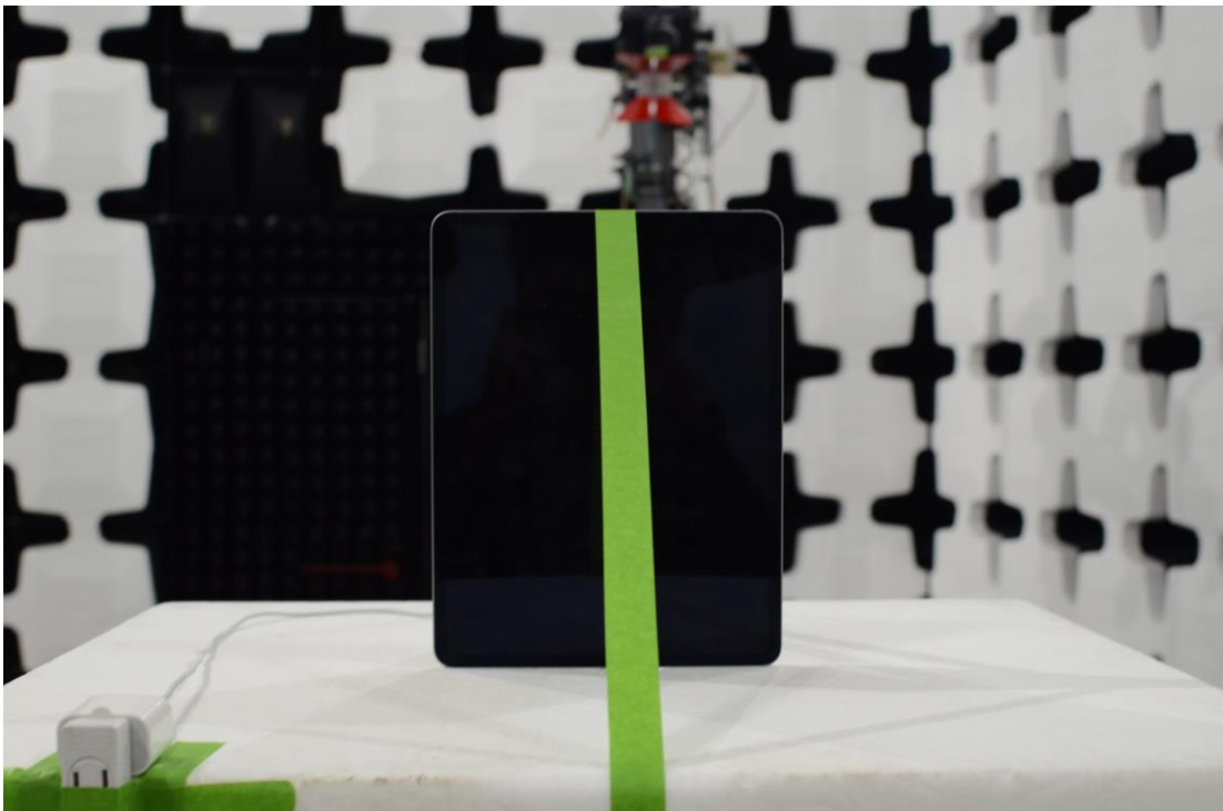
Figure 10: 1-18GHz Test Setup (Rear View)
