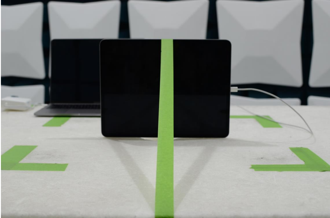
Figure 19: 30MHz-1GHz Test Setup (Front View)
