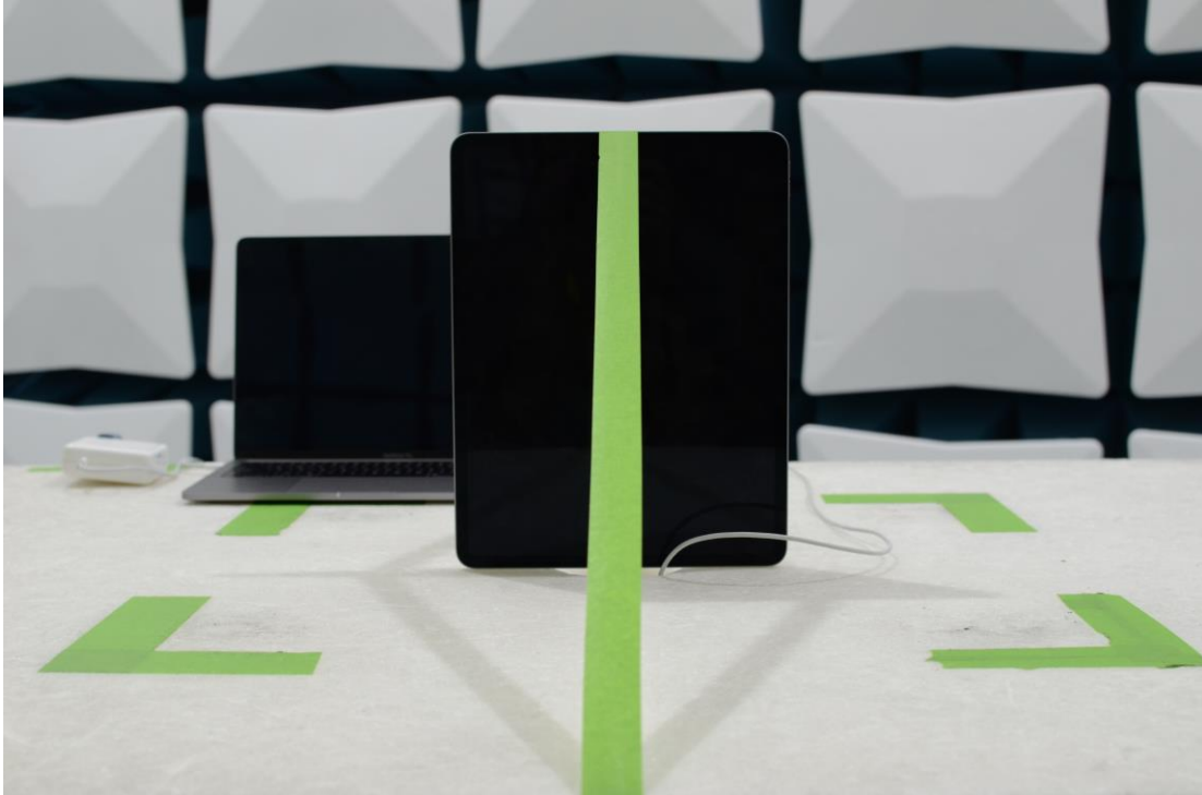
Figure 21: 30MHz-1GHz Test Setup (Front View)
