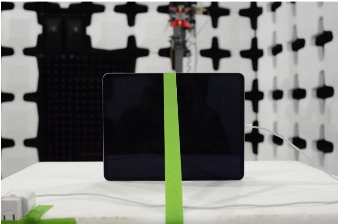
Figure 8: 1-18GHz Test Setup (Rear View)
