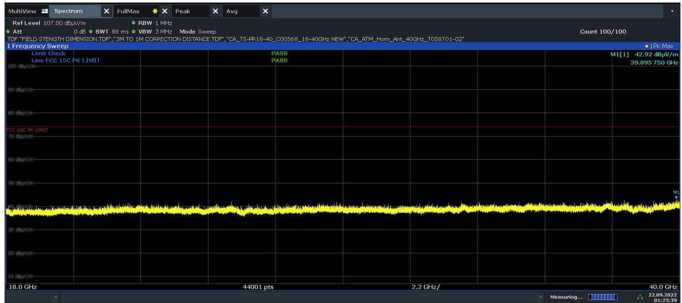
Plot 7-66. Radiated Spurious Emissions Above 18GHz TxBF (BT GFSK – 2480 MHz, Pol H)
