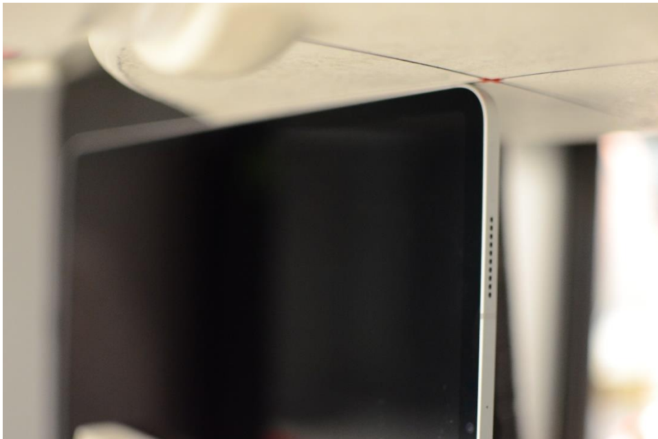
SAR Test Setup Photo 8 Left Edge at 0mm, Antennas WF7, WF8
