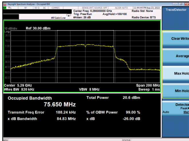
Plot 7-101. 26dB BW & 99% OBW Antenna WF5b (80MHz BW 802.11ac – Ch. 58, MCS4)
