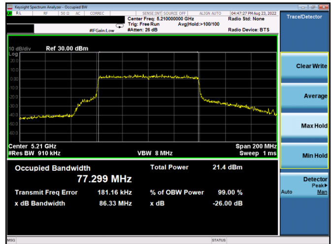
Plot 7-72. 26dB BW & 99% OBW Antenna WF5b (80MHz BW 802.11ax(SU) – Ch. 42, MCS2)
