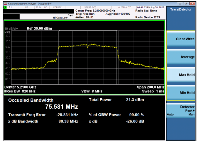
Plot 7-27. 26dB BW & 99% OBW Antenna WF5t (80MHz BW 802.11ac – Ch. 42, MCS4)
