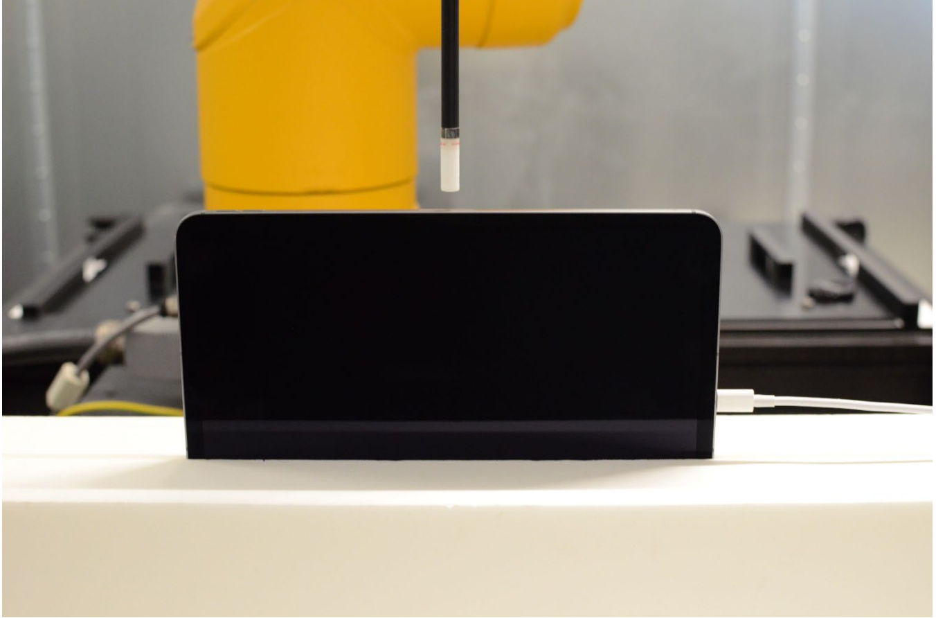
Figure G-11 Near Field Power Density Test Setup Photo – Right Edge at 8.58 mm
