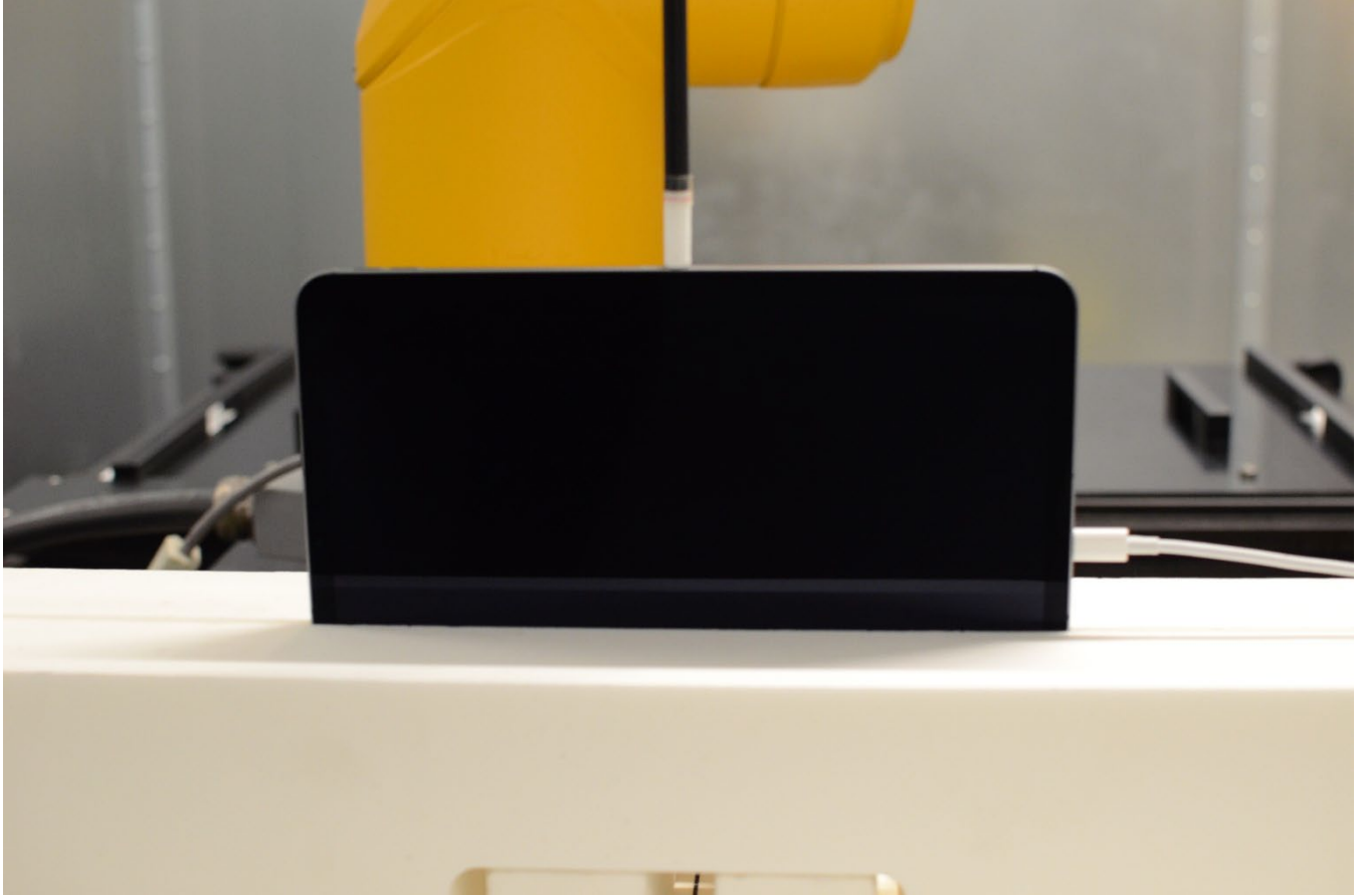
Figure G-10 Near Field Power Density Test Setup Photo – Right Edge at 2 mm
