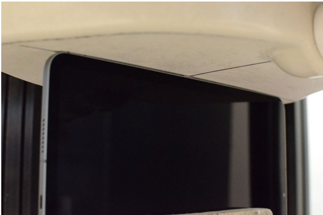
Figure G-8 SAR Test Setup Photo – Left Edge at 0mm
