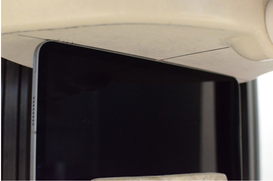
Figure G-7 SAR Test Setup Photo – Right Edge at 0 mm
