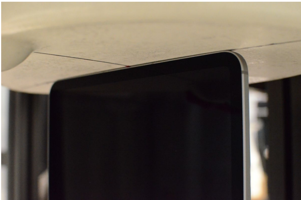
Figure G-6 SAR Test Setup Photo – Bottom Edge at 0 mm
