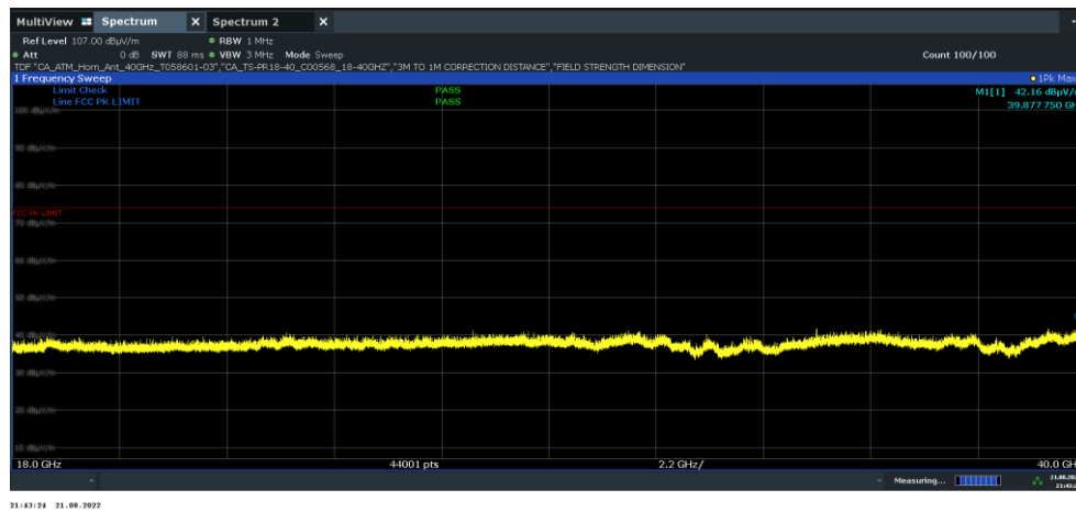
Plot 7-759. Radiated Spurious Emissions 18-40GHz SDM (802.11ax – Ch. 1 – RU26, Pol. H)
