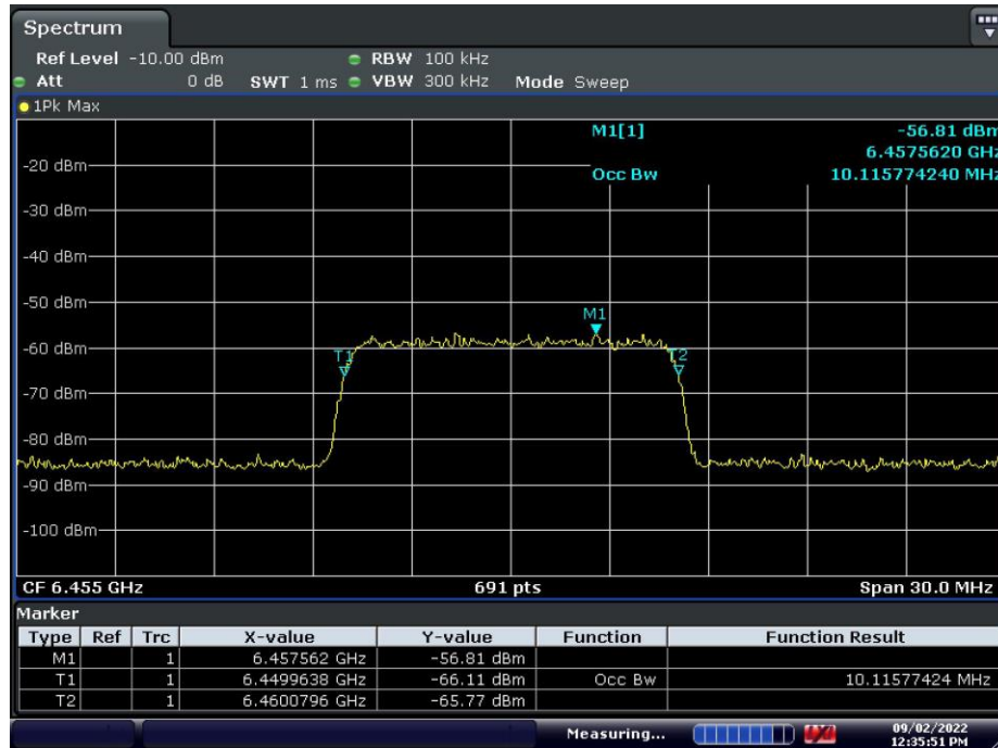
Plot 7-645. AWGN Signal – UNII 6 – 20MHz
