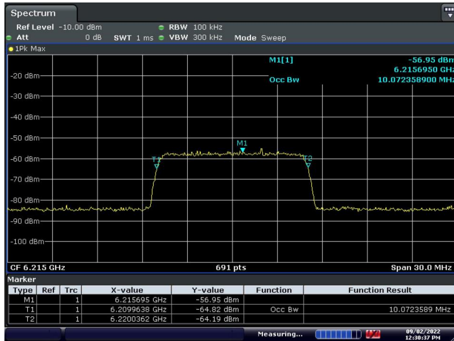
Plot 7-641. AWGN Signal – UNII 5 – 20MHz
