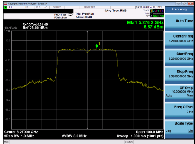
Plot 7-224. PSD Antenna 5b (40MHz BW 802.11ax(SU) – Ch. 54, MCS11)
