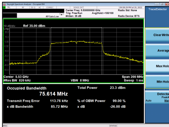
Plot 7-19. 26dB BW & 99% OBW Antenna 5b (80MHz BW 802.11ac – Ch. 106, MCS2)
