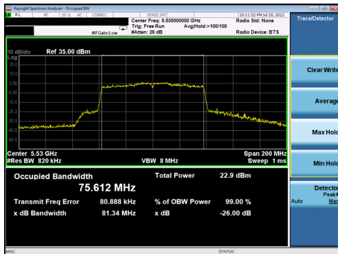
Plot 7-41. 26dB BW & 99% OBW Antenna 5b (80MHz BW 802.11ac – Ch. 106, MCS4)
