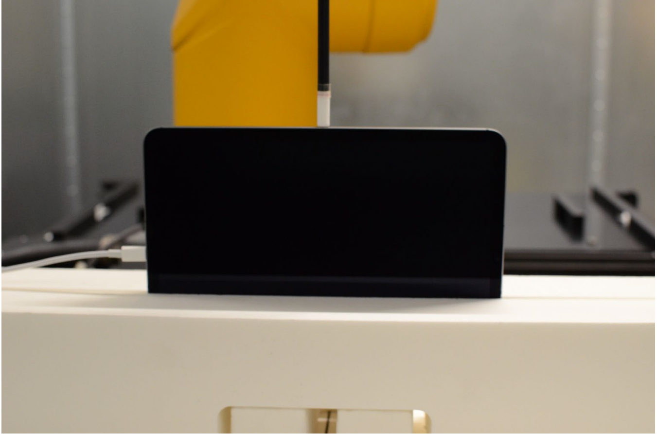
Figure G-12 Near Field Power Density Test Setup Photo – Left Edge at 2 mm
