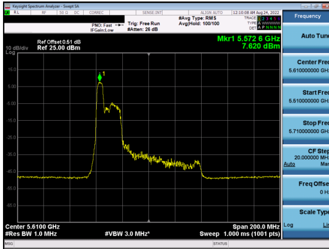
Plot 7-220. PSD Antenna WF5b (80MHz BW 11ax Index 37 – RU52 – Ch.122)
