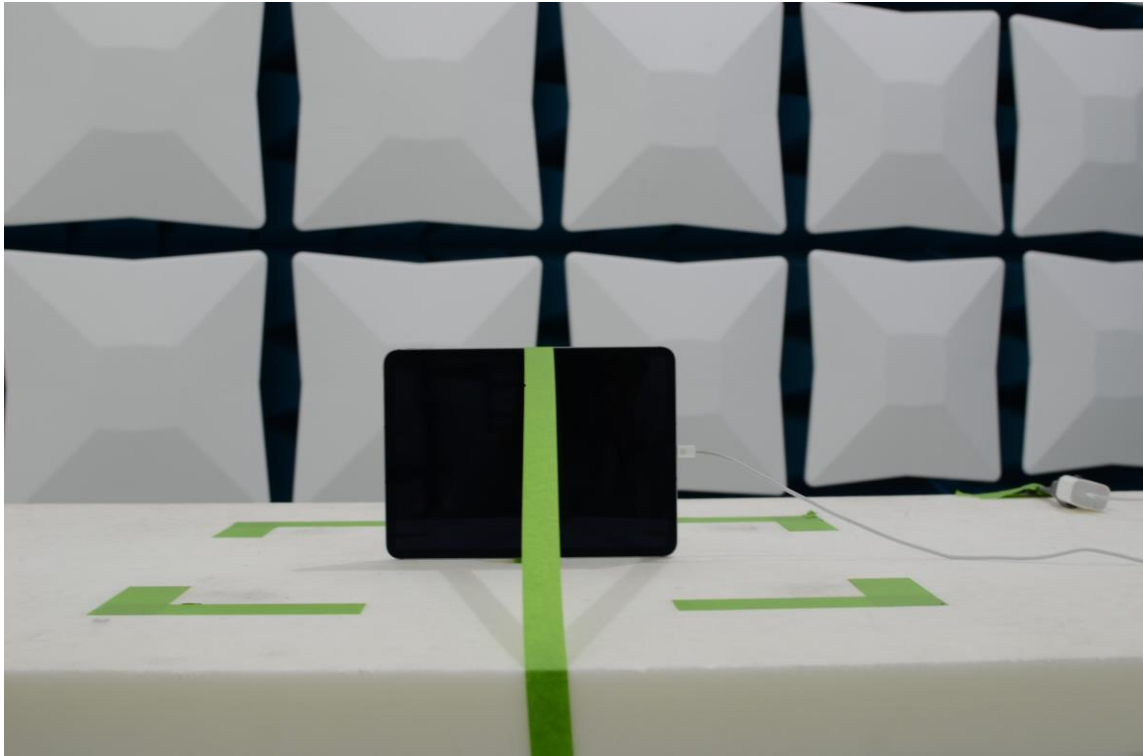
Figure 9: 30MHz-1GHz Test Setup (Front View)
