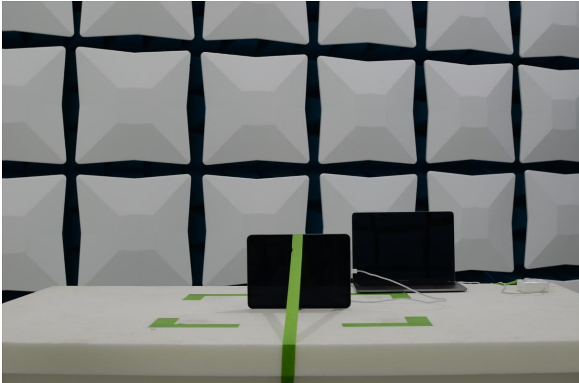
Figure 15: 30MHz-1GHz Test Setup (Front View)
