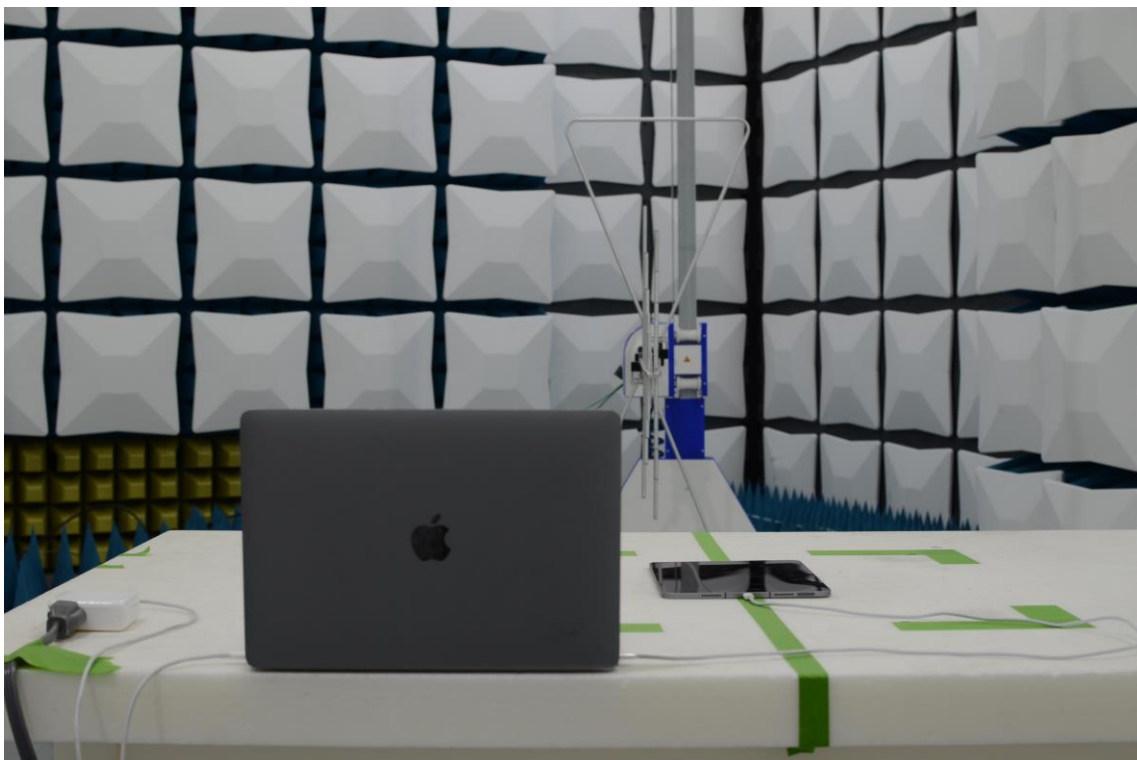
Figure 14: 30MHz-1GHz Test Setup (Rear View)
