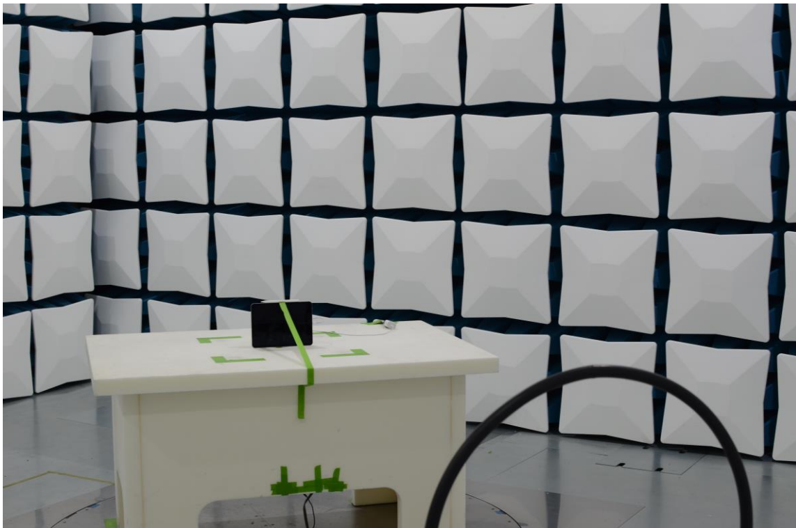
Figure 20: 9kHz-30MHz Test Setup (Front View)
