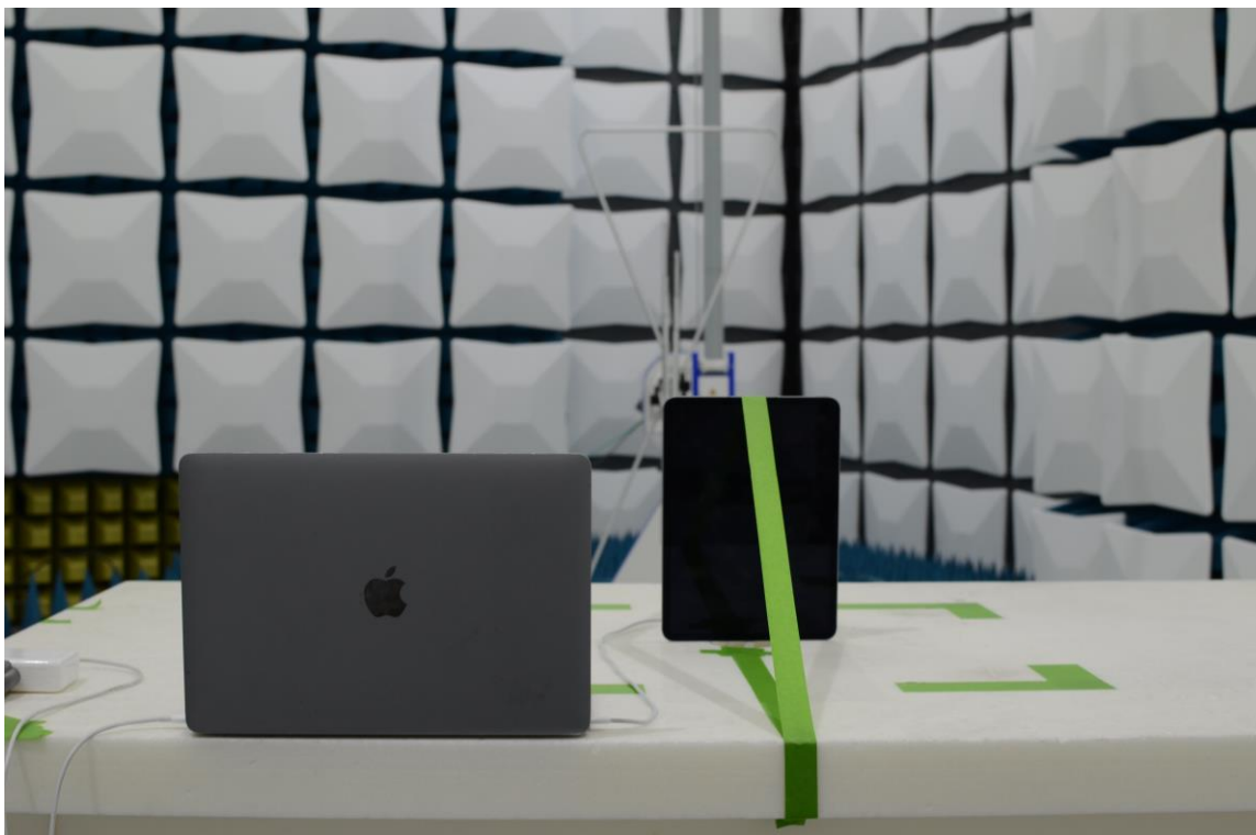
Figure 18: 30MHz-1GHz Test Setup (Rear View)
