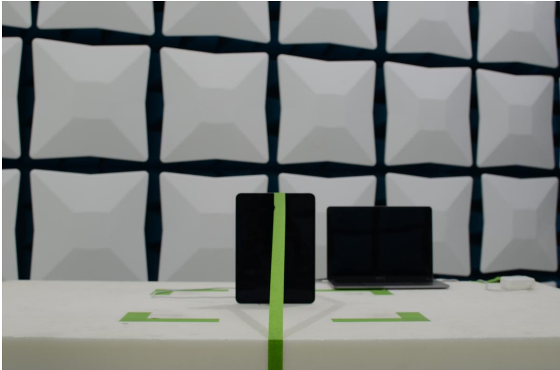
Figure 17: 30MHz-1GHz Test Setup (Front View)
