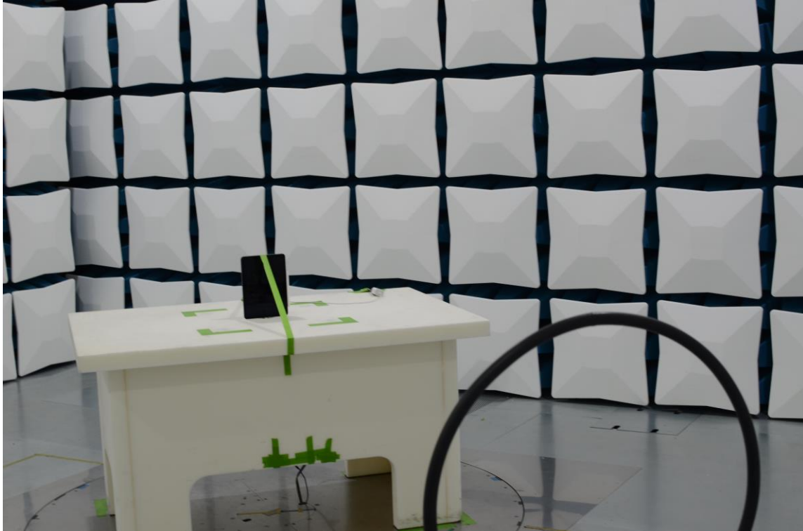
Figure 21: 9kHz-30MHz Test Setup (Front View)
