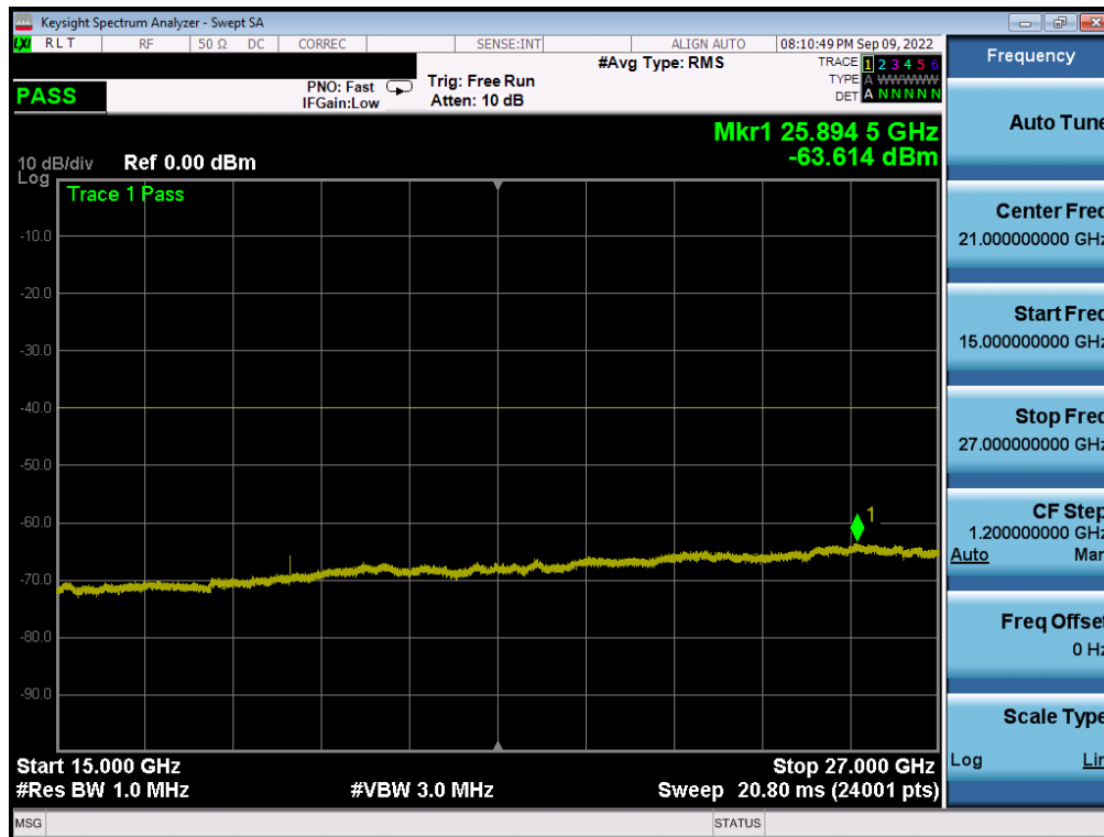
Plot 7-51. Conducted Spurious Plot (ULCA Band 48 - 20+20MHz QPSK - Mid Channel)
