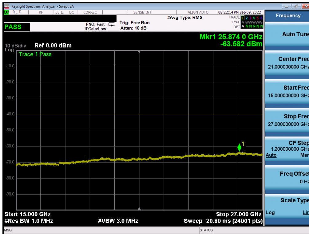
Plot 7-55. Conducted Spurious Plot (ULCA Band 48 - 20+20MHz QPSK - High Channel)
