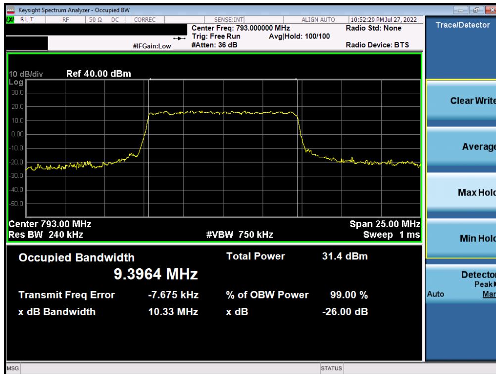
Plot 7-33. Occupied Bandwidth Plot (NR Band 14 - 10MHz CP-OFDM 64-QAM - Full RB Configuration)
