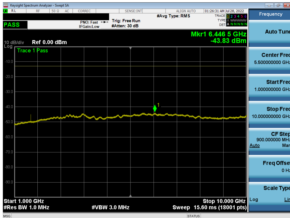
Plot 7-50. Conducted Spurious Plot (LTE Band 26 - 10MHz QPSK - RB Size 1, RB Offset 0 - Mid Channel)
