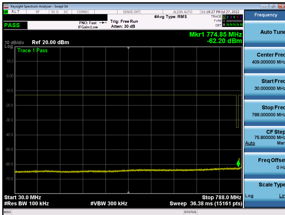
Plot 7-66. Conducted Spurious Plot (NR Band n14 - 10MHz DFT-s-OFDM QPSK - RB Size 1, RB Offset 0 – Mid Channel)
