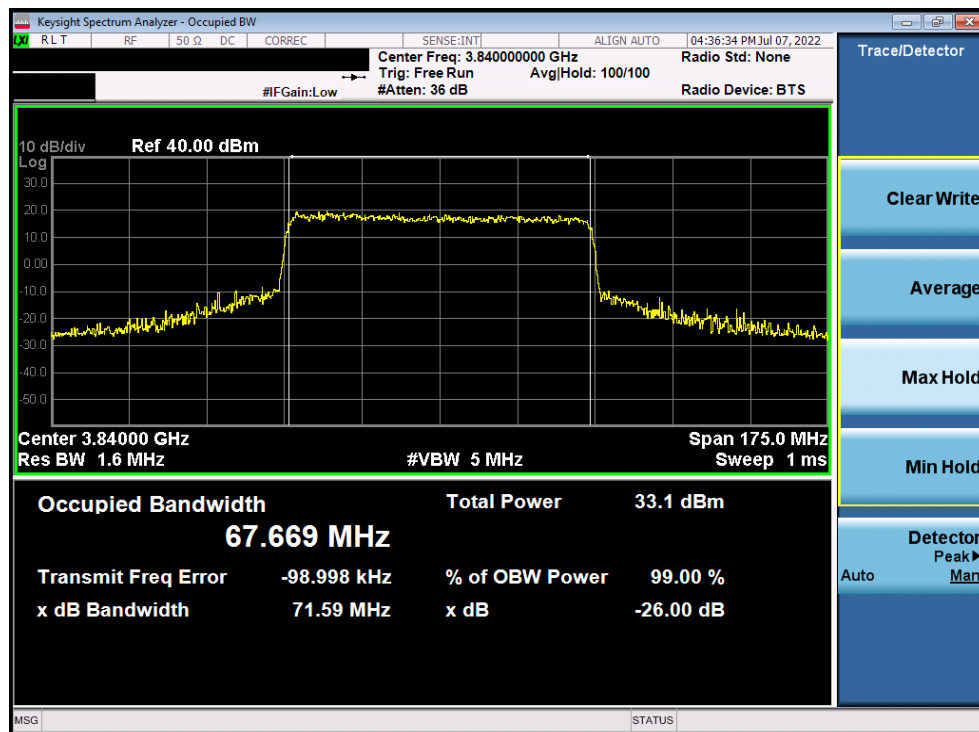
Plot 7-93. Occupied Bandwidth Plot (NR Band n77 C-Band - 70MHz CP-OFDM 16-QAM - Full RB)
