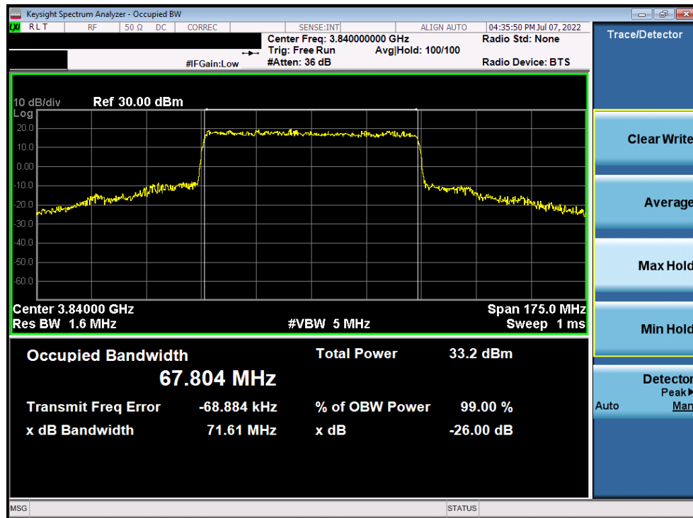
Plot 7-94. Occupied Bandwidth Plot (NR Band n77 C-Band - 70MHz CP-OFDM 64-QAM - Full RB)
