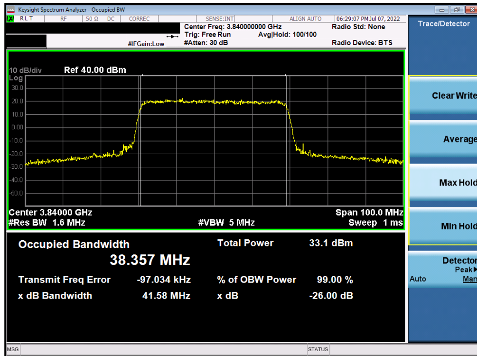
Plot 7-78. Occupied Bandwidth Plot (NR Band n77 C-Band - 40MHz CP-OFDM 16-QAM - Full RB)
