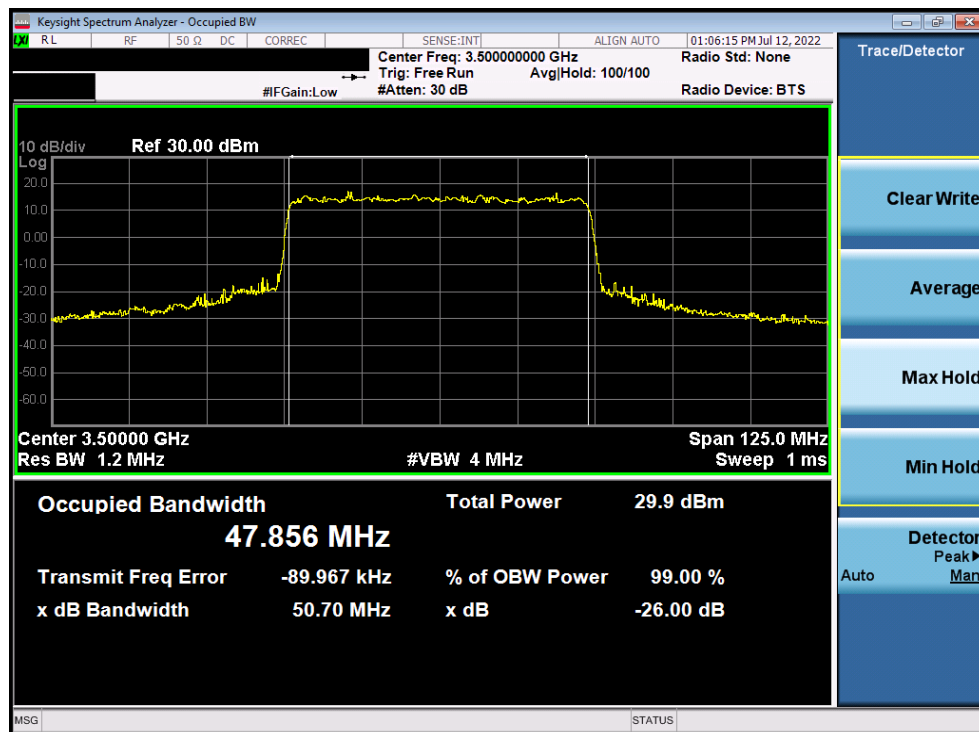
Plot 7-30. Occupied Bandwidth Plot (NR Band n77 DoD Band - 50MHz CP-OFDM 256-QAM - Full RB)
