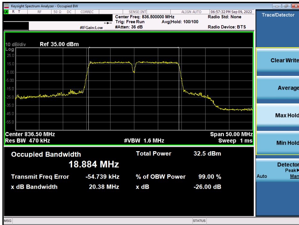
Plot 7-37. Occupied Bandwidth Plot (ULCA LTE Band 5 – (10 + 10)MHz QPSK - Full RB Configuration)
