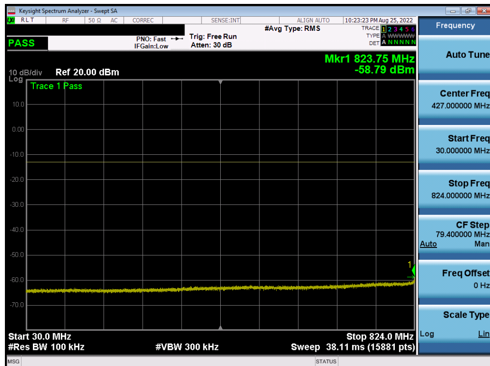
Plot 7-54. CSE (ULCA LTE Band 5 – (10 + 10)MHz QPSK – PCC 1/0 SCC 1/49 - High Channel)
