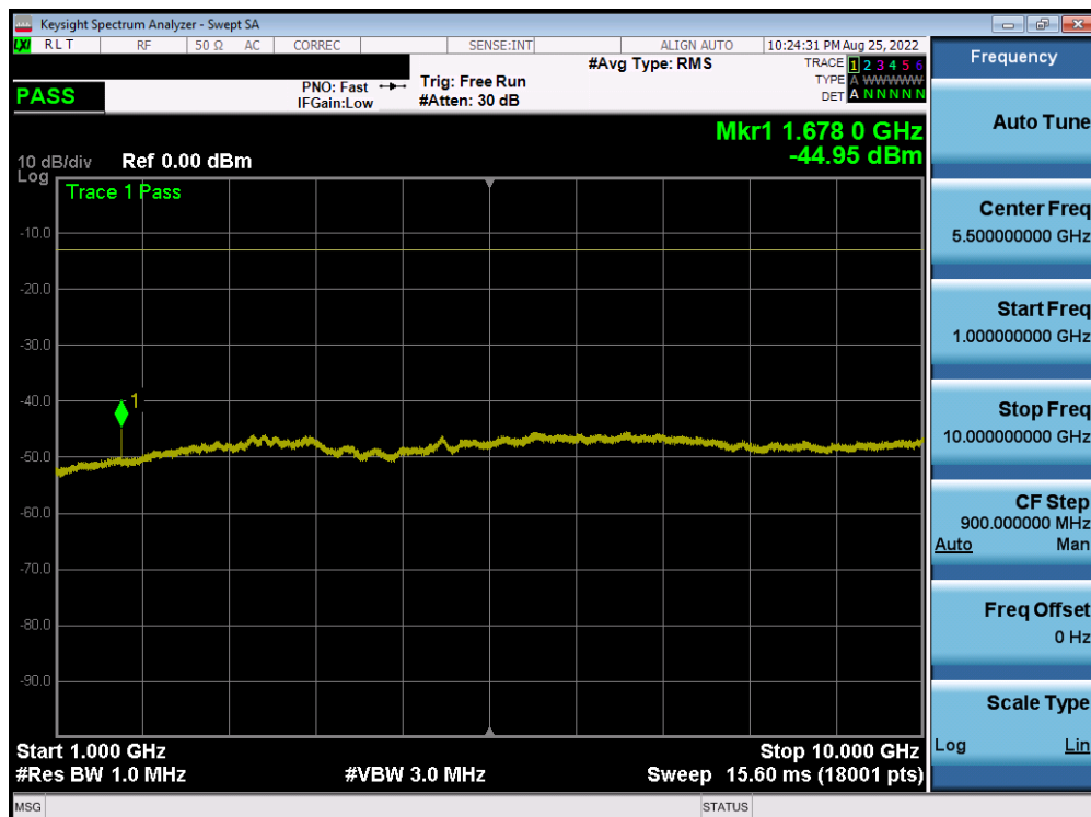
Plot 7-56. CSE (ULCA LTE Band 5 – (10 + 10)MHz QPSK – PCC 1/0 SCC 1/49 - High Channel)
