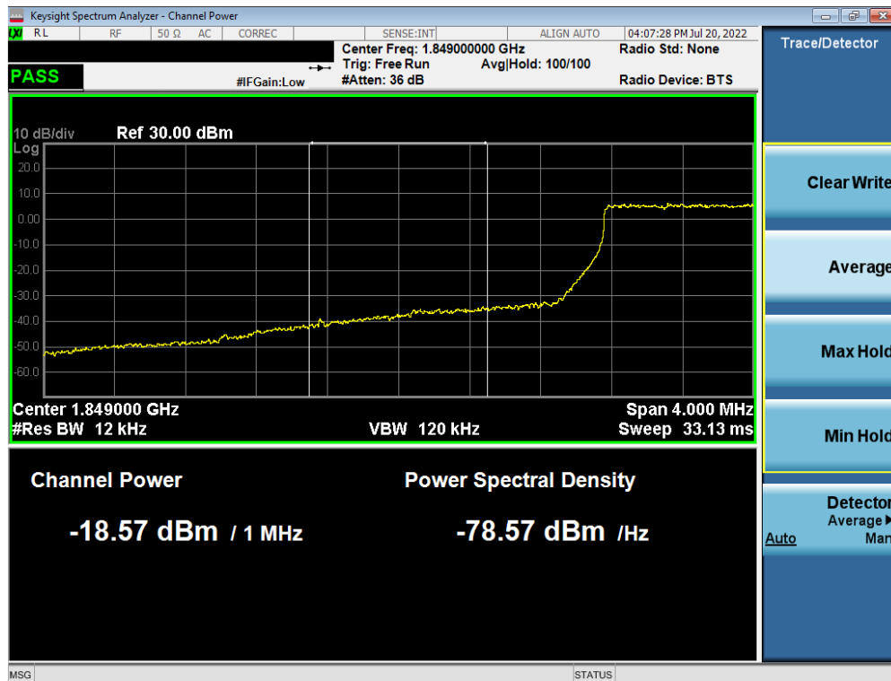
Plot 7-113. Extended Lower Band Edge Plot (LTE Band 2 – 1.4MHz QPSK – Full RB Configuration)
