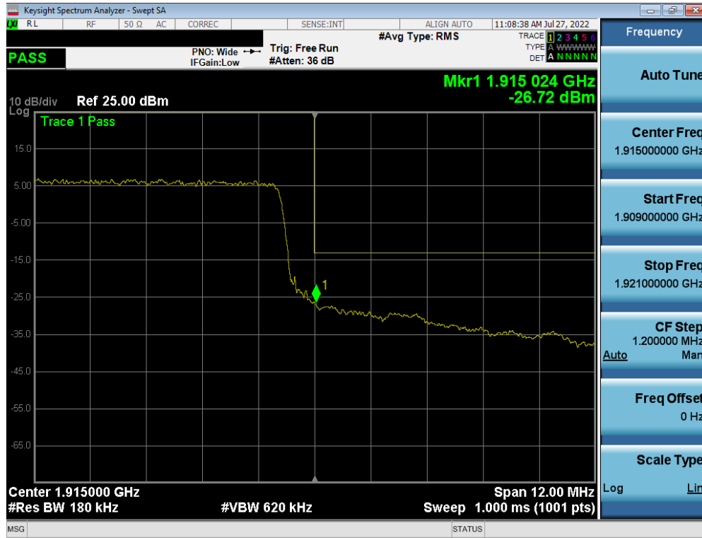
Plot 7-106. Upper Band Edge Plot (LTE Band 25 – 15MHz QPSK – Full RB Configuration)
