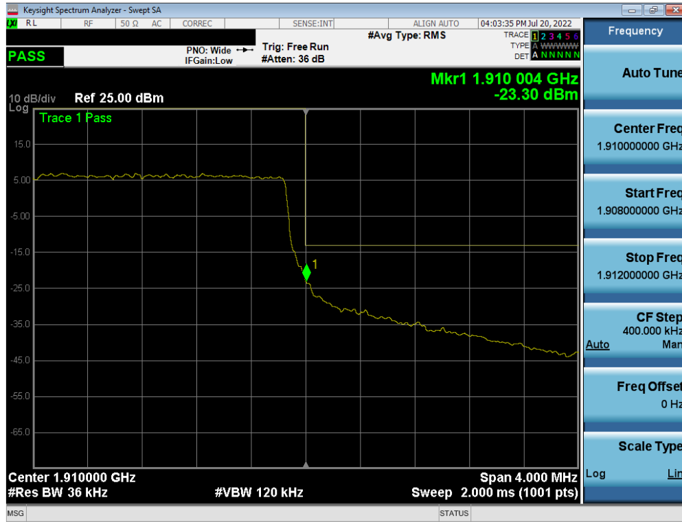
Plot 7-118. Upper Band Edge Plot (LTE Band 2 – 3MHz QPSK – Full RB Configuration)
