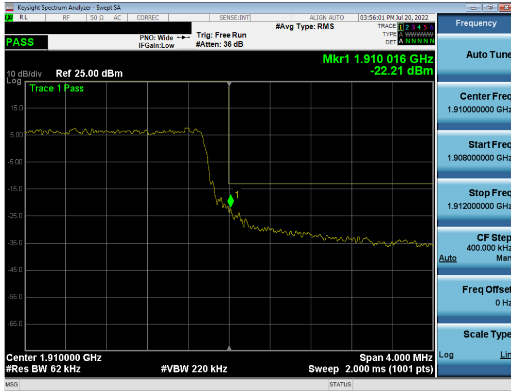
Plot 7-122. Upper Band Edge Plot (LTE Band 2 – 5MHz QPSK – Full RB Configuration)
