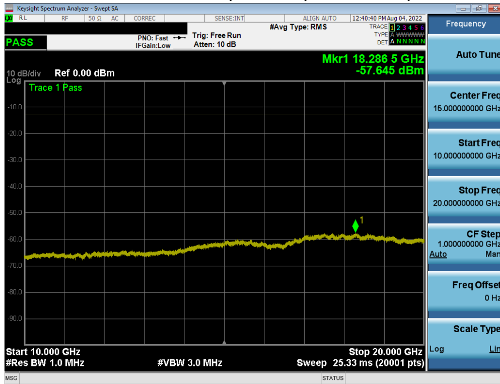
Plot 7-81. Conducted Spurious Plot (WCDMA Ch. 9262)
