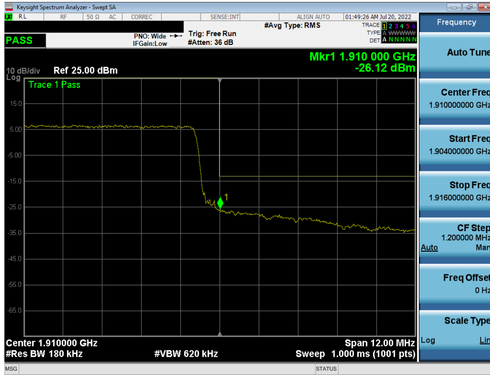
Plot 7-130. Upper Band Edge Plot (LTE Band 2 – 15MHz QPSK – Full RB Configuration)
