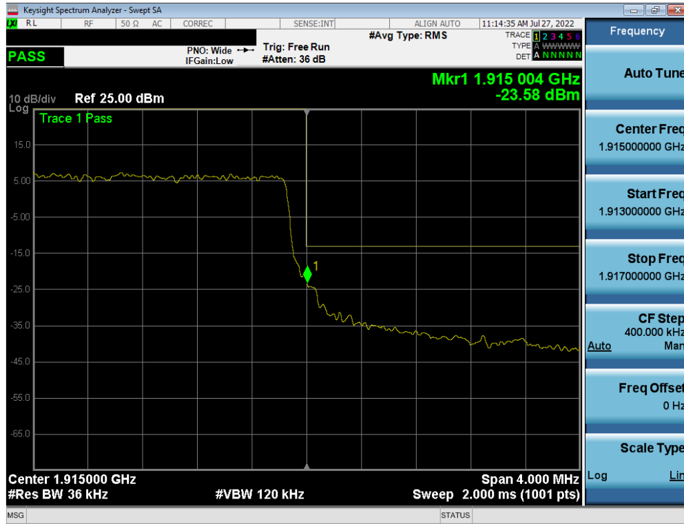
Plot 7-94. Upper Band Edge Plot (LTE Band 25 – 3MHz QPSK – Full RB Configuration)
