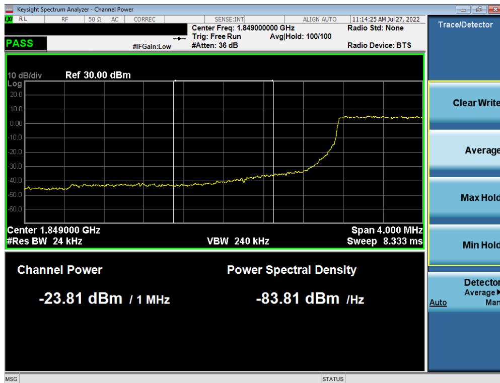
Plot 7-93. Extended Lower Band Edge Plot (LTE Band 25 – 3MHz QPSK – Full RB Configuration)
