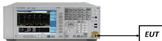
Figure 7-5. Radiated Measurement Setup
