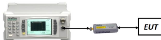
Figure 7-2. Radiated Measurement Setup for Power Meter Measurements
