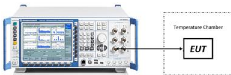
Figure 7-8. Test Instrument & Measurement Setup
