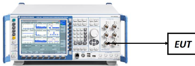
Figure 7-4. Conducted Power Measurement Setup
