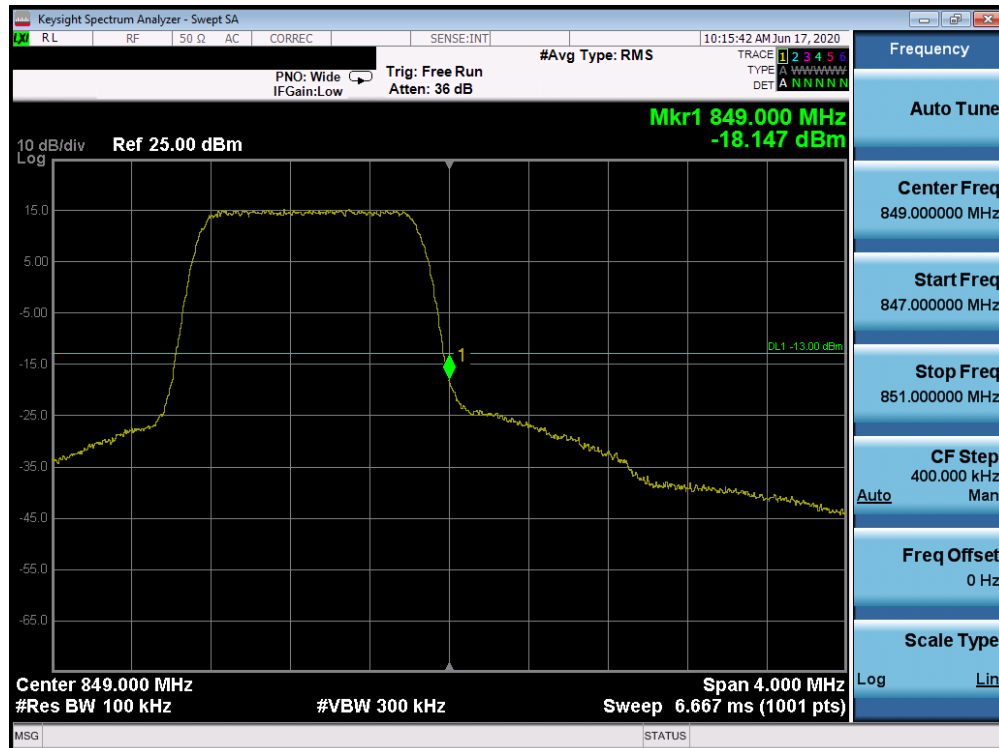
Plot 7-190. Upper Band Edge Plot (Band 26 - 1.4MHz QPSK - Full RB Configuration)
