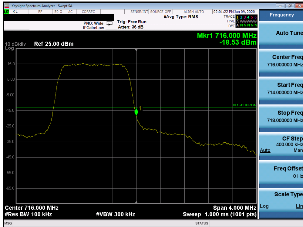
Plot 7-170. Upper Band Edge Plot (Band 12 - 1.4MHz QPSK - Full RB Configuration)
