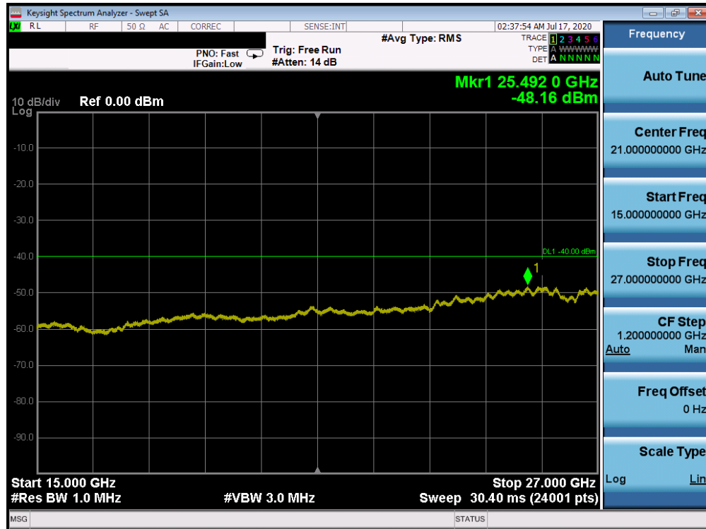
Plot 7-150. Conducted Spurious Plot (Band 30 - 5.0MHz QPSK - RB Size 1, RB Offset 0 - High Channel)
