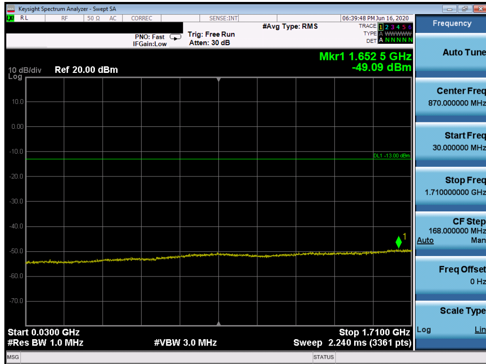
Plot 7-130. Conducted Spurious Plot (Band 66/4 - 20.0MHz QPSK - RB Size 1, RB Offset 0 - High Channel)
