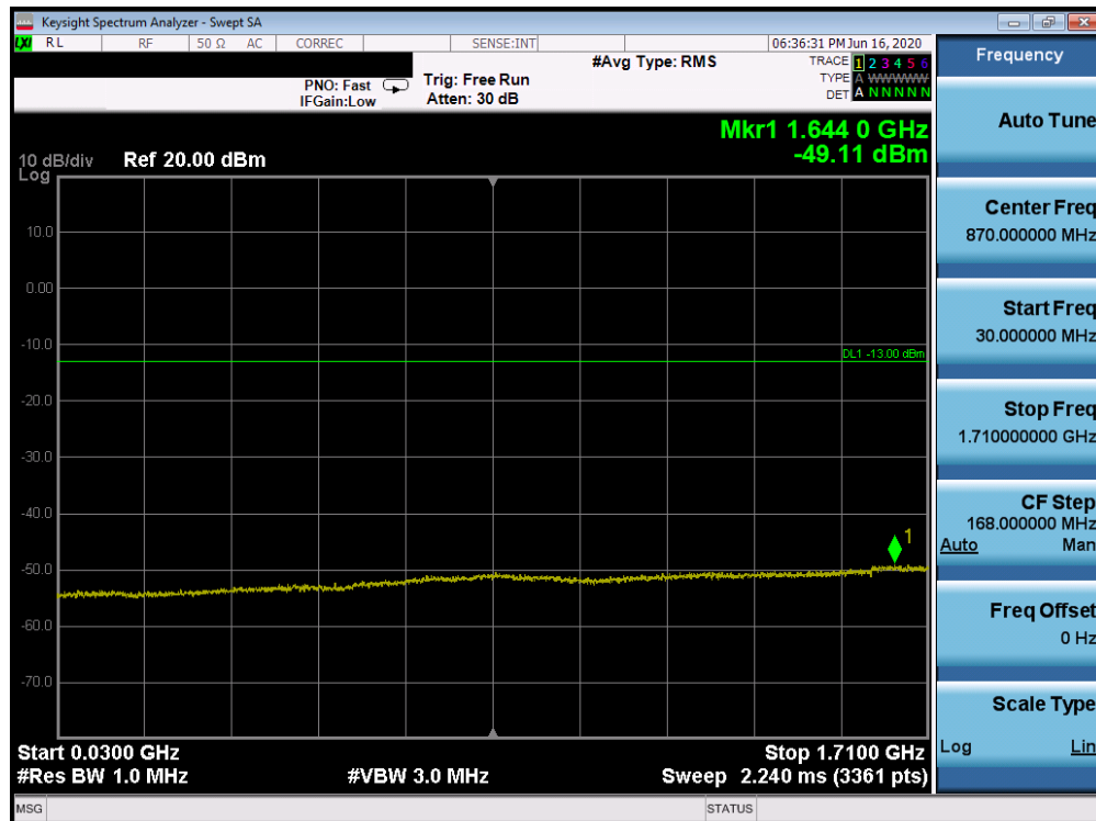
Plot 7-127. Conducted Spurious Plot (Band 66/4 - 20.0MHz QPSK - RB Size 1, RB Offset 0 - Mid Channel)
