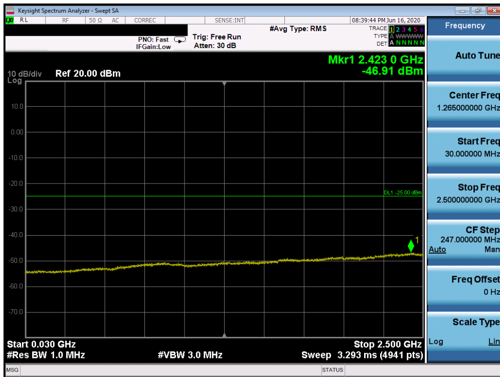
Plot 7-154. Conducted Spurious Plot (Band 7 - 20.0MHz QPSK - RB Size 1, RB Offset 0 - Mid Channel)
