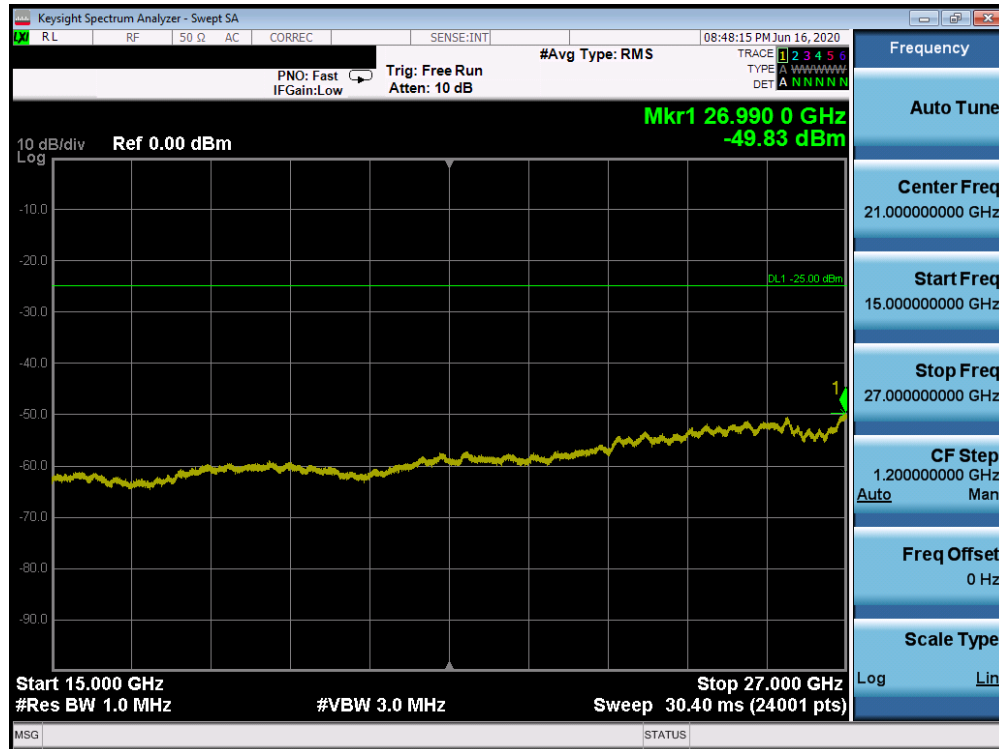
Plot 7-159. Conducted Spurious Plot (Band 7 - 20.0MHz QPSK - RB Size 1, RB Offset 0 - High Channel)
