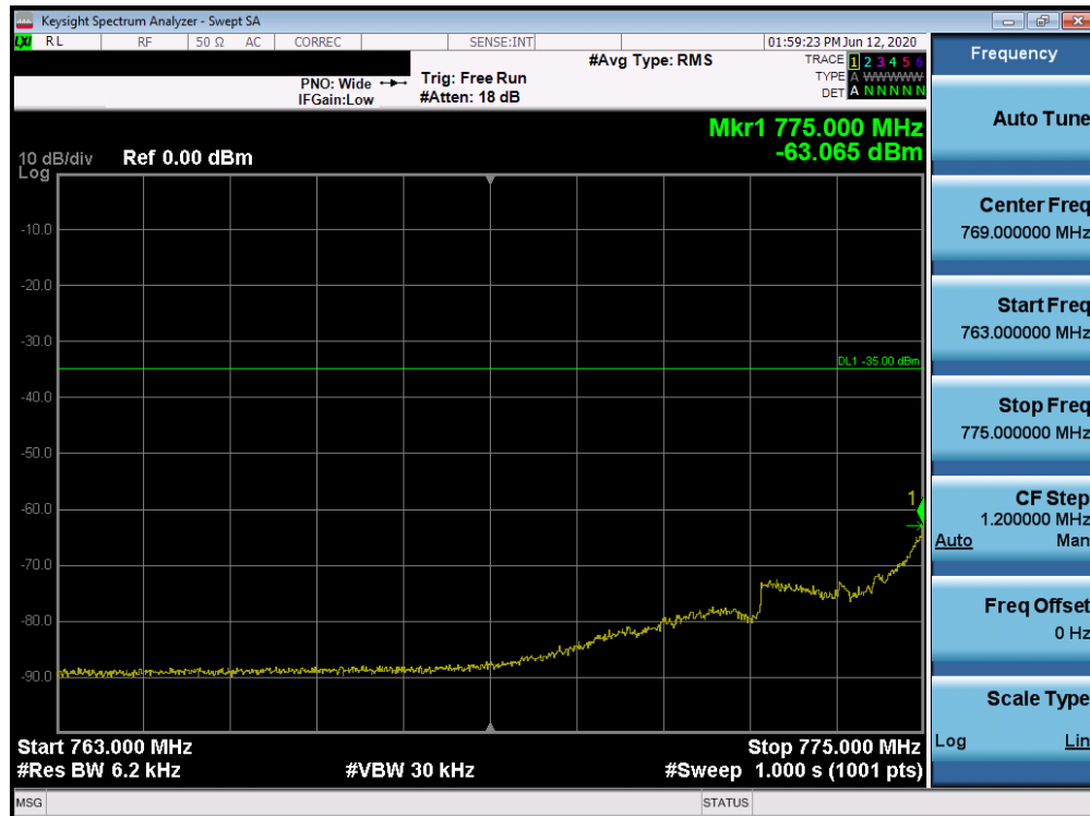
Plot 7-182. Lower Emission Mask Edge Plot (Band 13 - 5.0MHz QPSK - Full RB Configuration)
