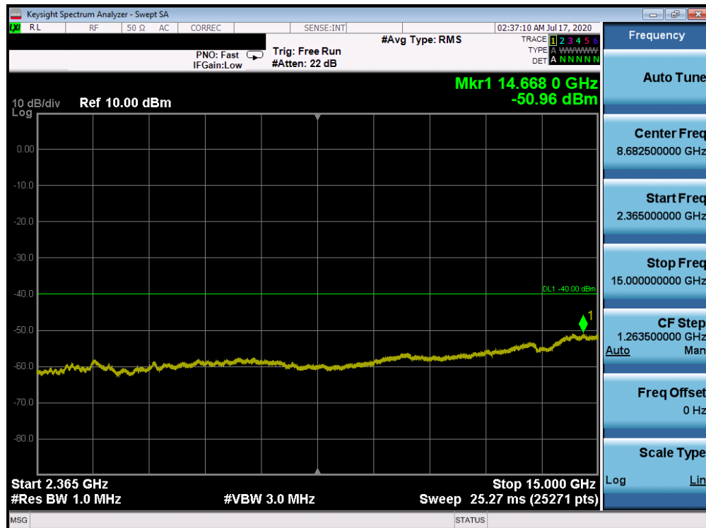
Plot 7-149. Conducted Spurious Plot (Band 30 - 5.0MHz QPSK - RB Size 1, RB Offset 0 - High Channel)
