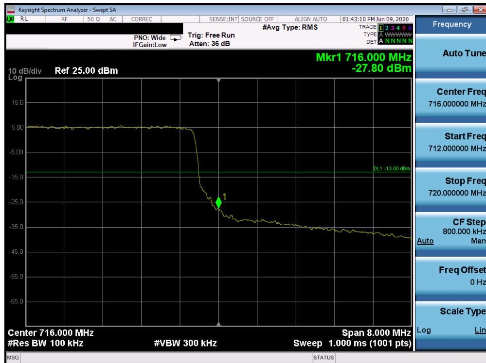
Plot 7-176. Upper Band Edge Plot (Band 12 - 10.0MHz QPSK - Full RB Configuration)
