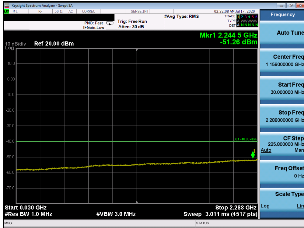
Plot 7-142. Conducted Spurious Plot (Band 30 - 5.0MHz QPSK - RB Size 1, RB Offset 0 - Low Channel)
