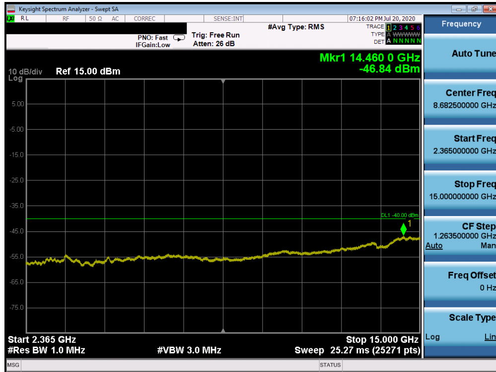
Plot 7-146. Conducted Spurious Plot (Band 30 - 10.0MHz QPSK - RB Size 1, RB Offset 0 - Mid Channel)
