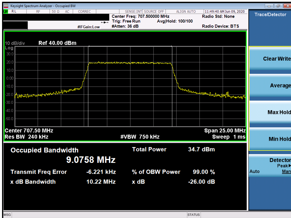
Plot 7-10. Occupied Bandwidth Plot (Band 12/17 - 10.0MHz QPSK - Full RB Configuration)
