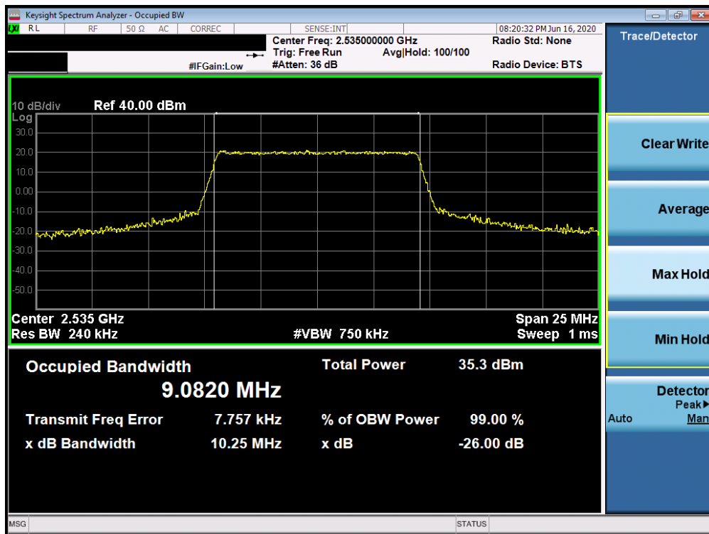
Plot 7-76. Occupied Bandwidth Plot (Band 7 - 10.0MHz QPSK - Full RB Configuration)
