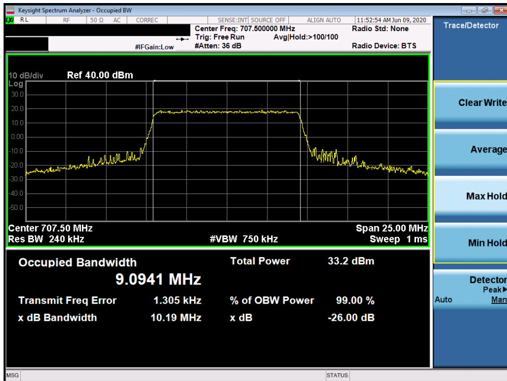
Plot 7-12. Occupied Bandwidth Plot (Band 12/17 - 10.0MHz 64-QAM - Full RB Configuration)
