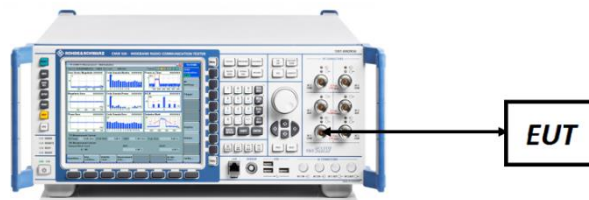
Figure 7-7. ERP/EIRP Measurement Setup
