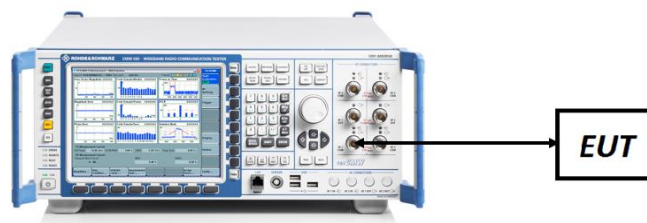
Figure 7-5. ERP/EIRP Measurement Setup
