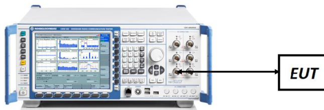
Figure 7-4. Conducted Power Measurement Setup
